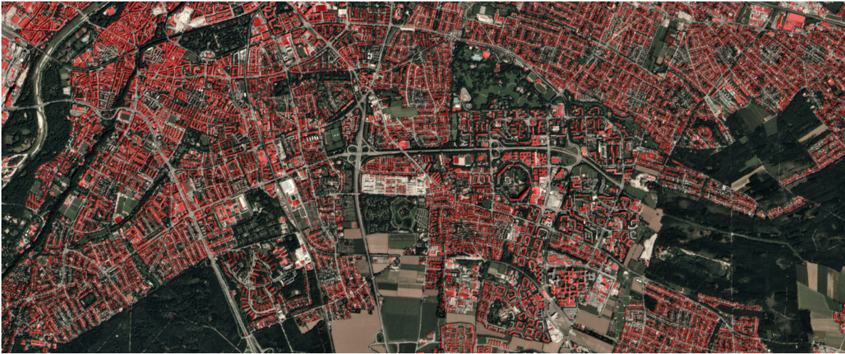
Fig. 6. Section of the entire Munich test area. Red color indicates the building footprint generated by the proposed method and overlays an optical image.
