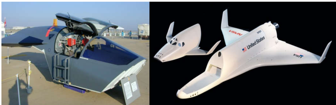
Fig. 3: F111 ejectable cabin part (left) and JSC Shuttle IIc with detachable crew compartment
