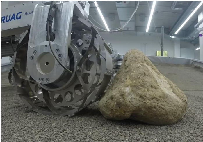
Figure 6.10: FR wheel climbing obstacle. Courtesy DLR.
