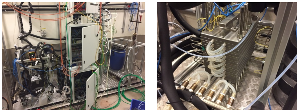
Fig. 6 [Left] Pilot plant for continuous titration. [Right] Continuous flow plate reactor.
