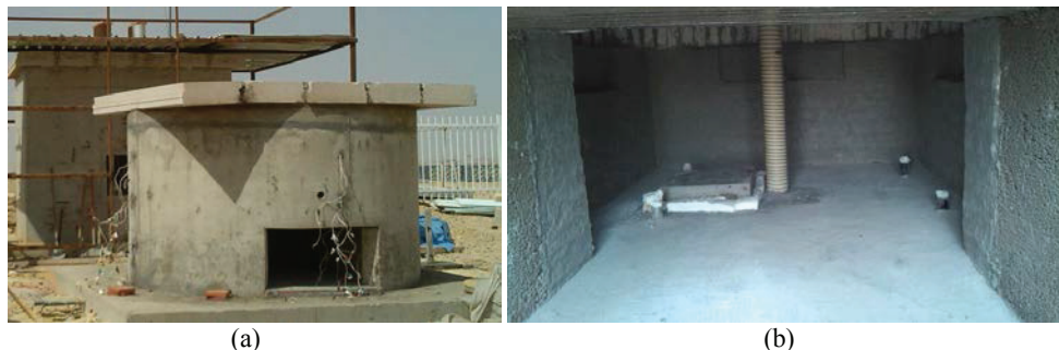
FIGURE 8. Ground-based cylindrical particle storage test facility: (a) overall view of the cylindrical bin, (b) the electric heater inserted along the centerline of the storage bin.
