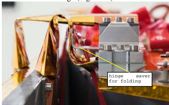
Figure 11. Hinges folded and brackets connected to the satellite. (hinges covered by SLI)
