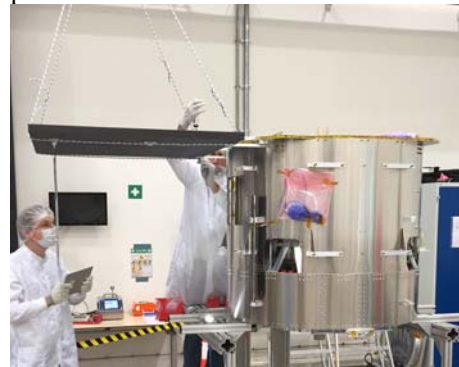
Figure 8. Installation of panels in the deployed state followed by folding of the panels.
