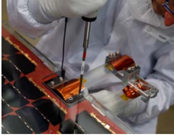
Figure 9. Pre installation of hinges with a bracket on the satellite side.
