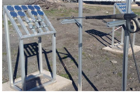
Fig. 2: Water jet cleaning setup.
