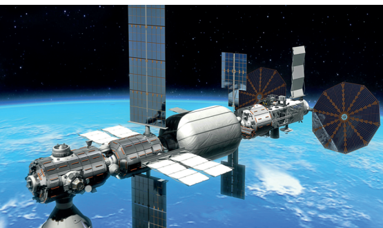
Figure 1: Illustration of DLR's Orbital Hub concept during the docked phase for servicing of the Free Flyer consisting of an external platform and a pressurised laboratory.
