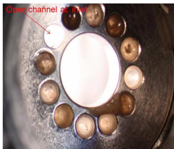
Fig 1. Biofilm formation inside the solenoid valve at the inlet to the International Space Station's Water Processor Mostly Liquid Separator (immediately downstream of the Water Processor Waste Tank). The image was taken by United Technologies Aerospace Systems (UTAS) during disassembly of the valve at the supplier facility (ValveTech, Inc) after the valve's return to Earth. Image: NASA.
