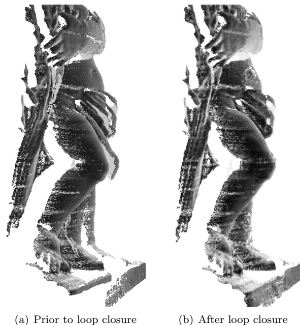
Figure 24: Pointcloud correction after successful loop closure.
