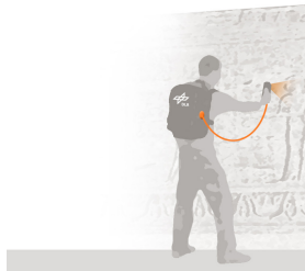
Figure 1: The portable DLR 3D-Modeler used for cultural heritage preservation.
