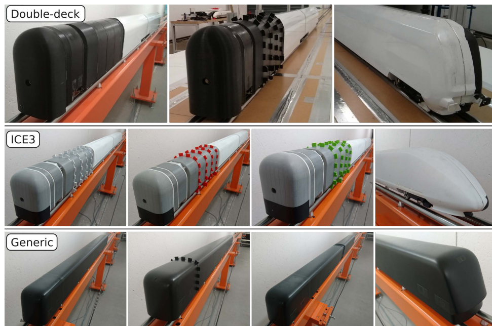
Figure 2: Train Models with a generic head shape in a smooth and rough surface configuration (left). The coaches have a simplified geometry of a double-deck train, an ICE3 and a generic train (right).
