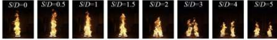
Fig. 3. Snapshots of flame shape with increasing S under D=13 cm.
