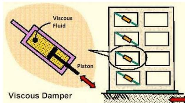
*Figure 1-1 viscous damper utilizes the forced movement of fluid within damper [28]*
