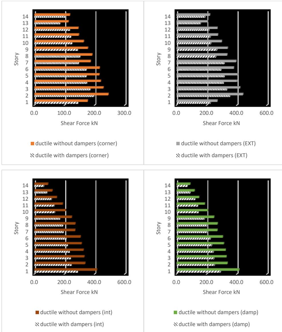
Figure 3-8 Shear Force columns comparisons between model (DUC) & (DUC-D): (a) between corner columns (b) between external columns (c) between internal columns (DUC) between internal columns connected to a damper
