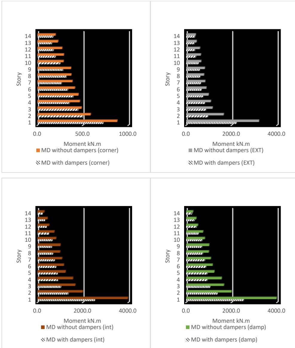
Figure 3-5 moment columns comparisons between model (MD) & (MD-D): (a) between corner columns (b) between external columns (c) between internal columns (DUC) between internal columns connected to dampers.
