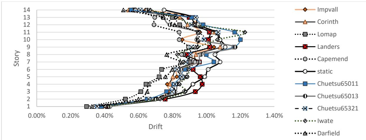
Figure 4-12 Time History drift for elastic with dampers model (EL-D)
