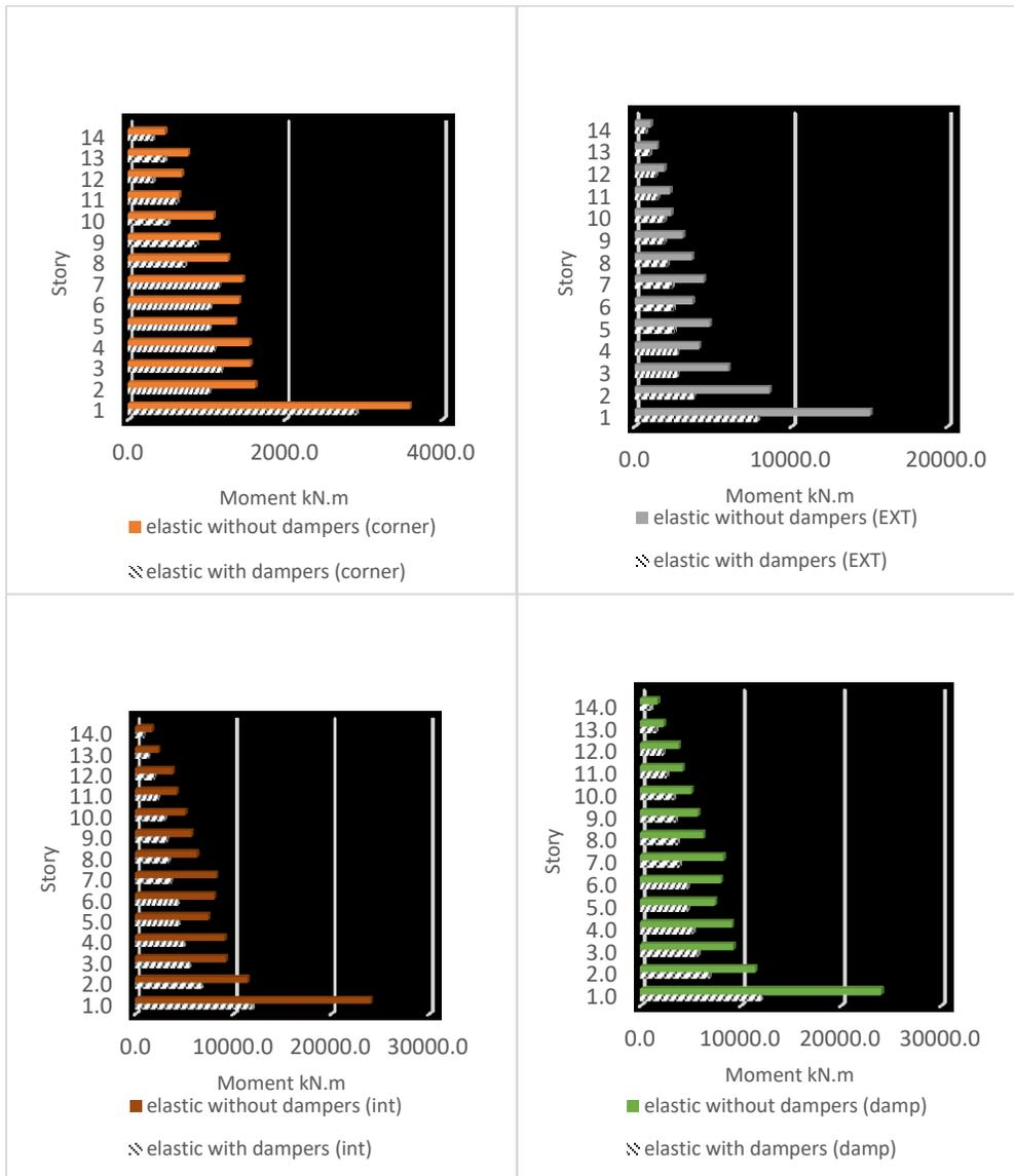
Figure 3-3 moment columns comparisons between model (EL) & (EL-D): (a) between corner columns (b) between external columns (c) between internal columns (DUC) between internal columns connected to a dampers
