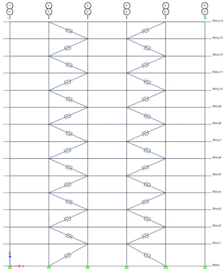
Figure 2-4 Frames views with dampers position
