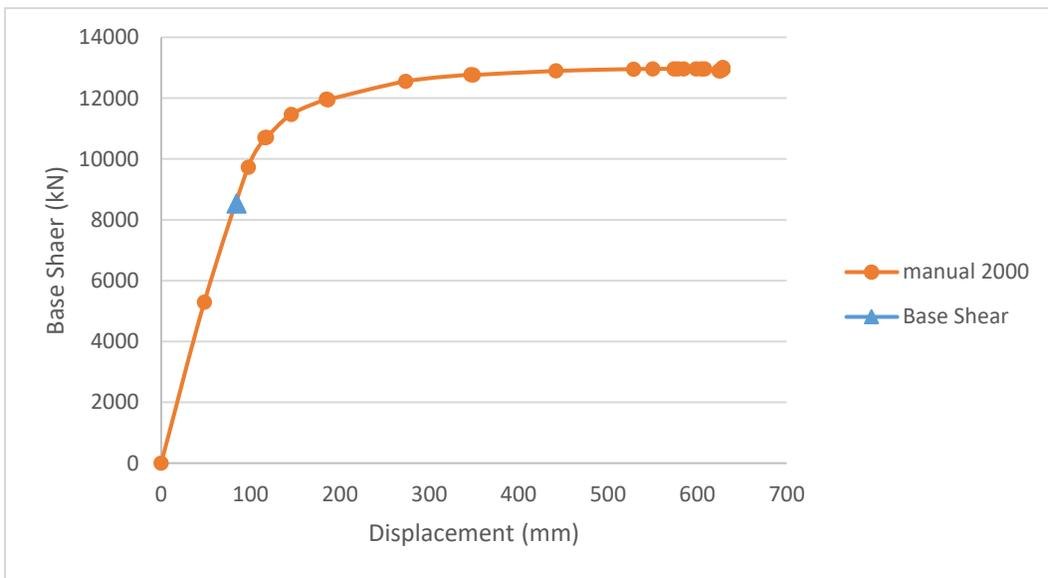
Figure 4-5 Push-Over curve for Moderately-Ductile with dampers building (MD-D)
