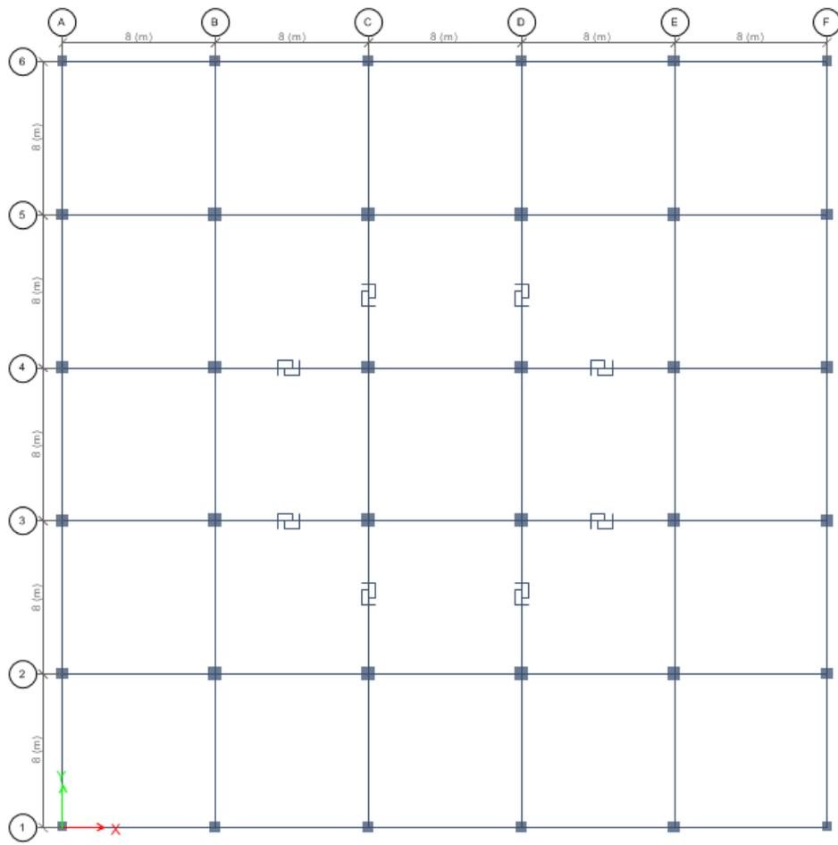
Figure 2-3 plans view with dampers
