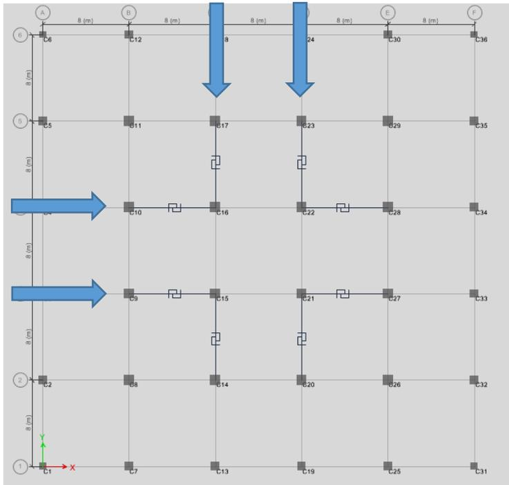
Figure 2-5 Floor view and dampers directions
