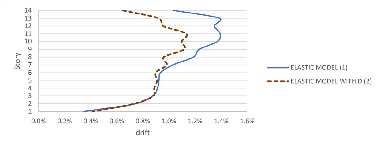
Figure 4-14 Standard deviation + Mean value Drift for time History analysis model (EL) & (EL-D)
