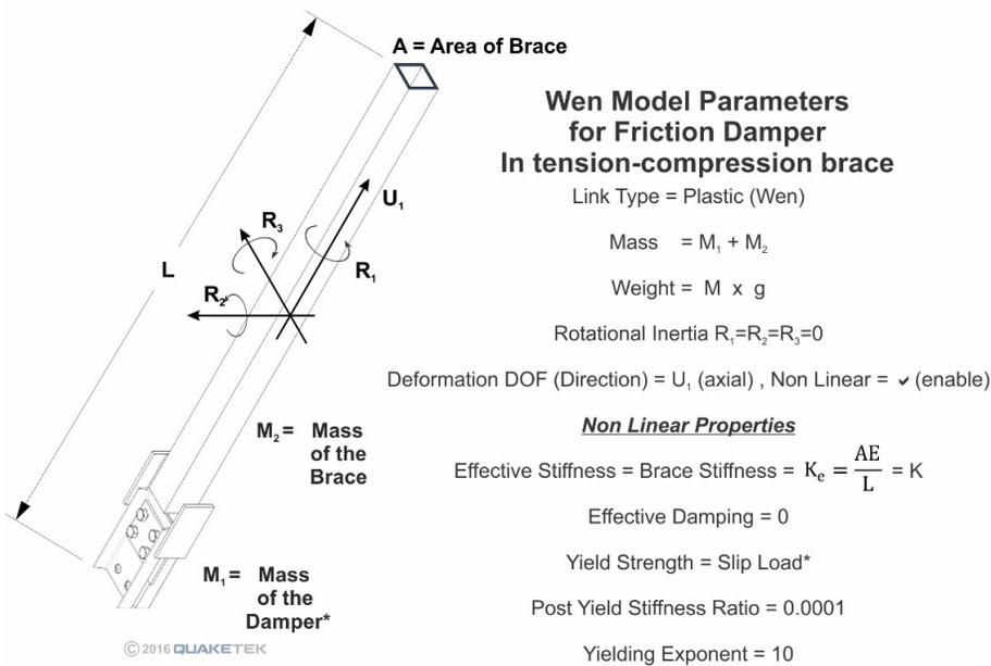
Figure 2-6 Wen Model parameters for Friction Dampers in tension-compression braces
