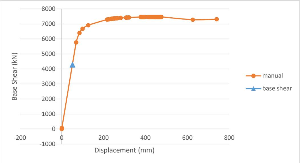
Figure 4-8 Pushover curve for ductile with damper building (DUC-D)
