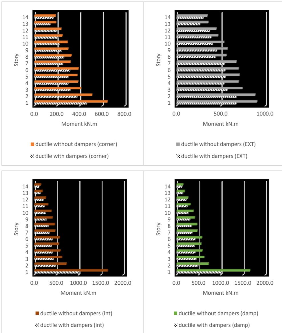
Figure 3-7 moment columns comparisons between model (DUC) & (DUC-D): (a) between corner columns (b) between external columns (c) between internal columns (DUC) between internal columns connected to a dampers.
