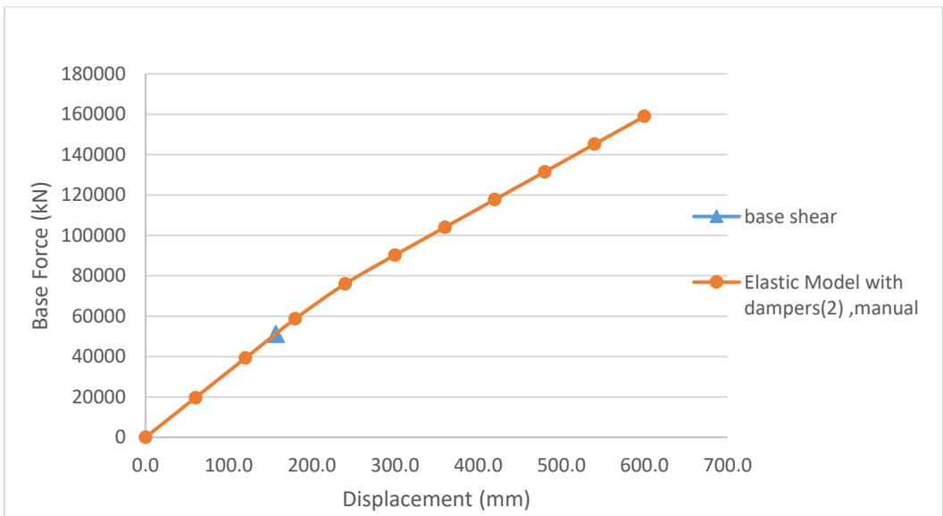
Figure 4-2 Pushover curve for Elastic with dampers building (EL-D)
