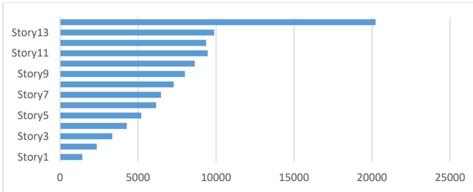
Figure 3-1 Lateral load applied on model (EL)
