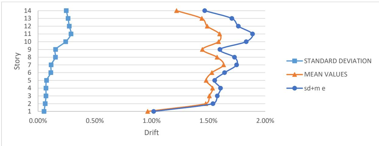
Figure 4-23 Standard deviation, mean values and sum for the Time History drift for ductile model with dampers (DUC-D)
