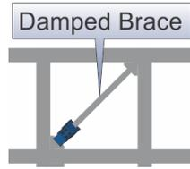
Figure 3-2 Damped brace included into a frame
