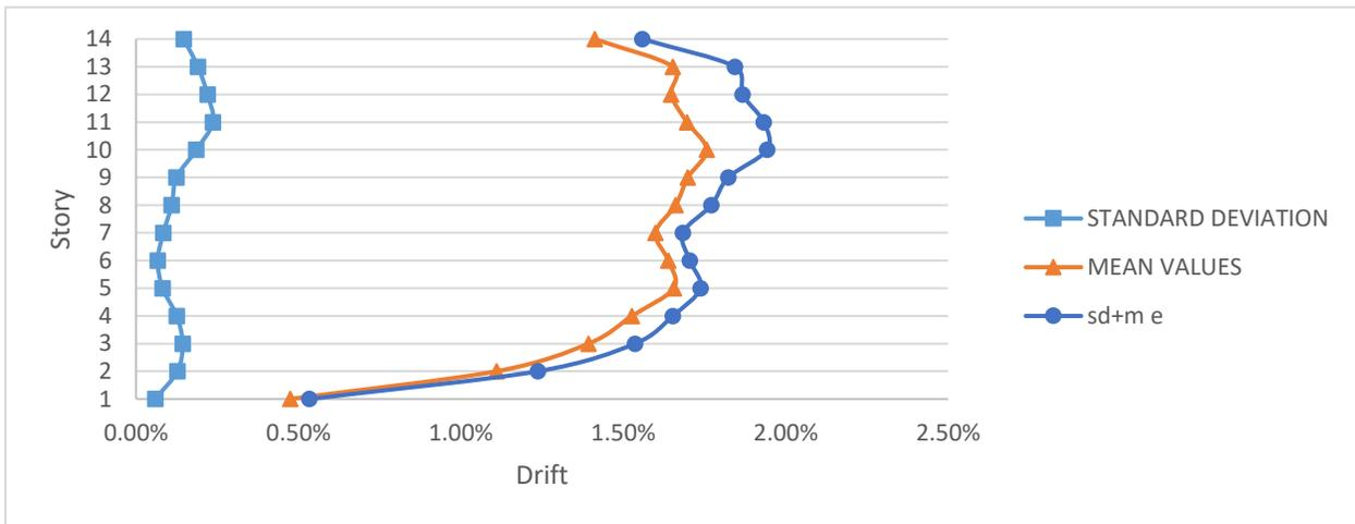
Figure 4-16 Standard deviation, mean values and sum for the Time History drift for moderately-ductile model (MD)
