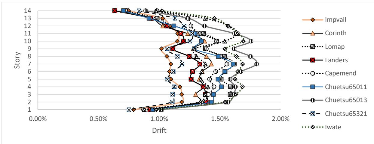
Figure 4-20 Time History drift for ductile model (DUC)
