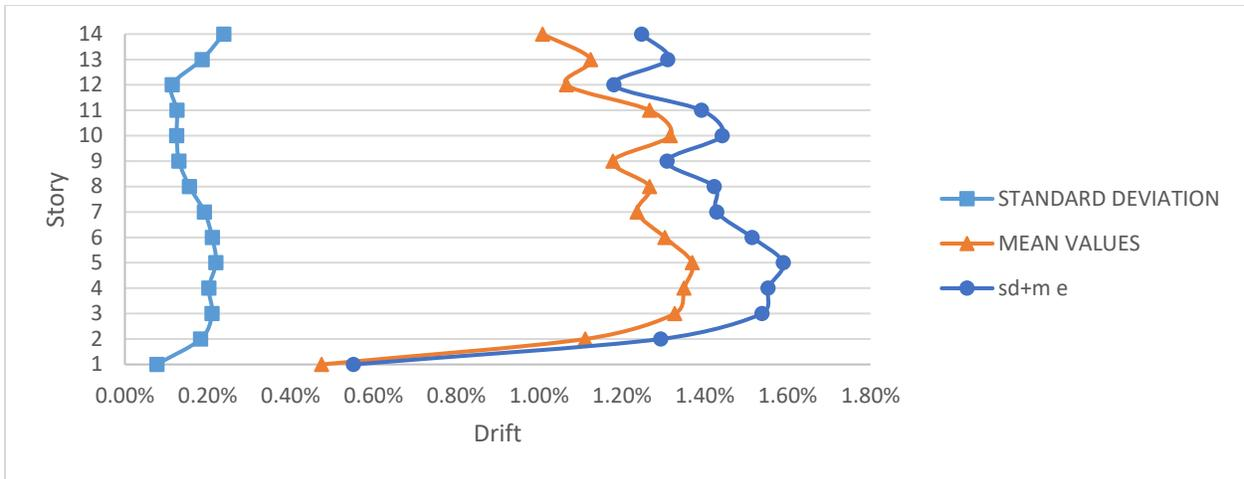
Figure 4-18 Standard deviation, mean values and sum for the Time History drift for moderately-ductile model with dampers (MD-D)
