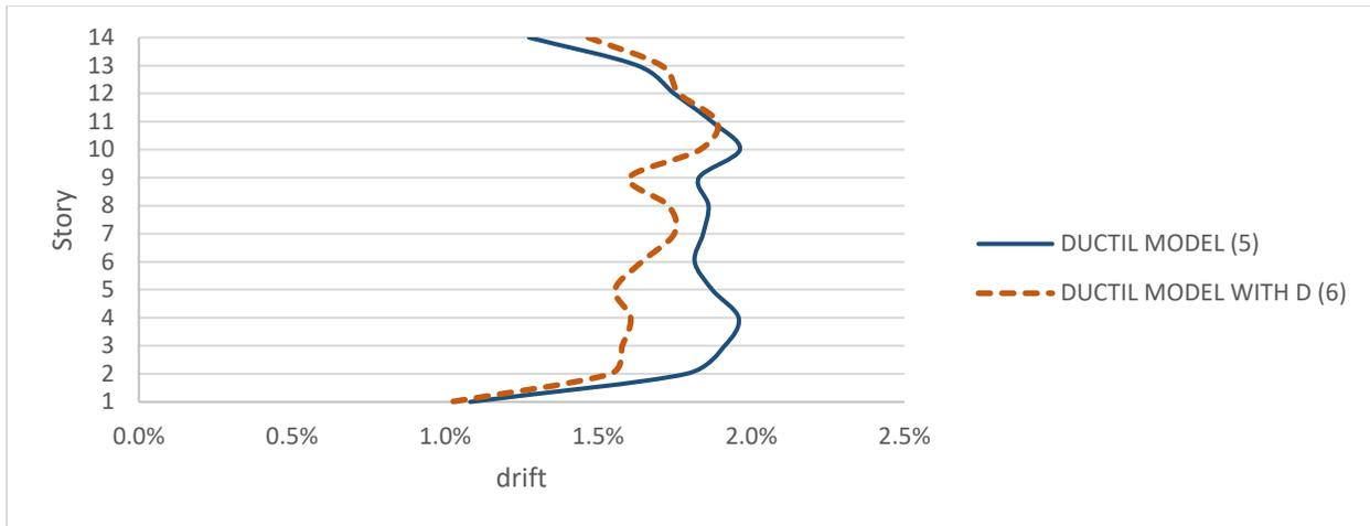
Figure 4-24 Standard deviation + Mean value Drift for time History analysis model (DUC) & (DUC-D)
