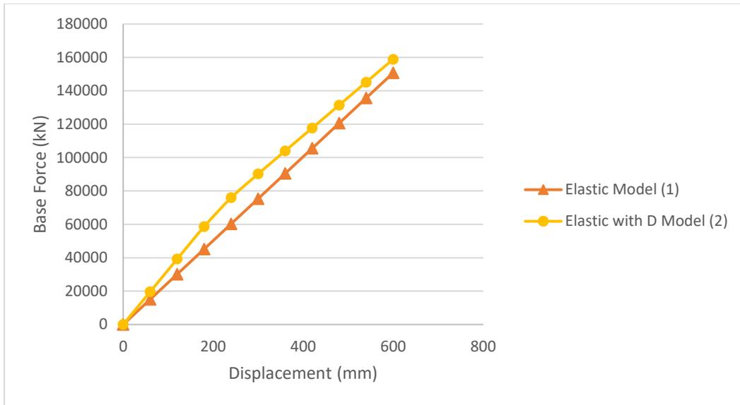
Figure 4-3 Pushover curve for Elastic building (EL) & (EL-D)
