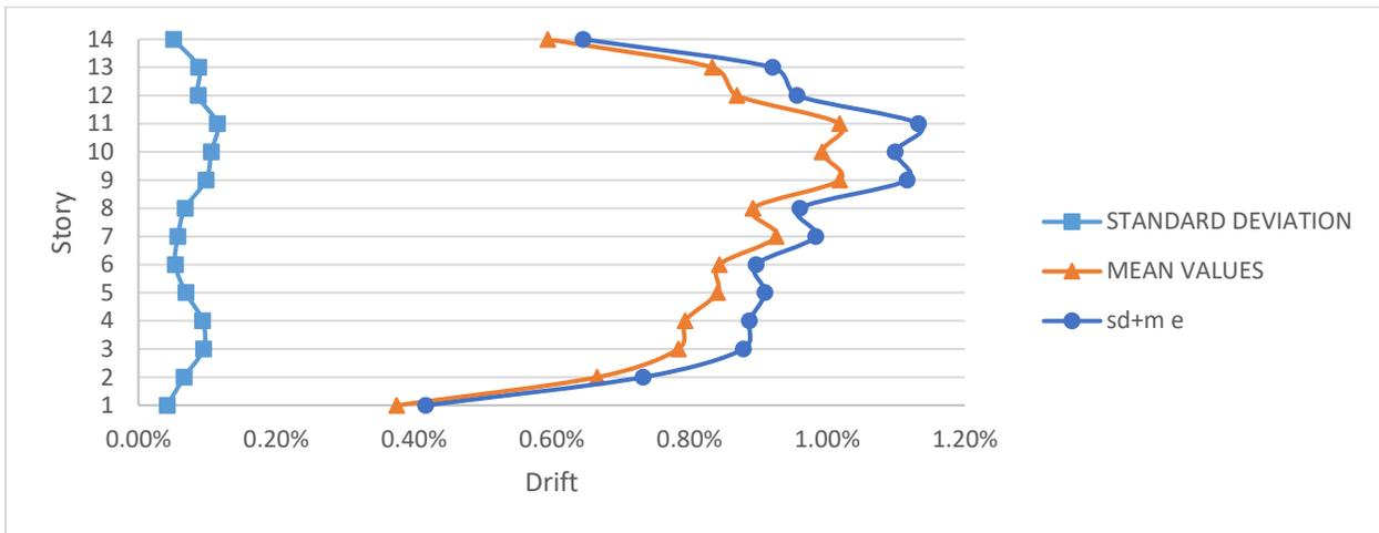
Figure 4-13 Standard deviation, mean values and sum for the Time History drift for elastic model with dampers (EL-D)
