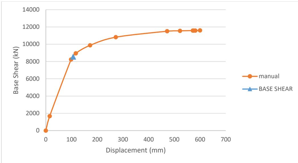
Figure 4-4 Push-Over curve for Moderately-Ductile building (MD)
