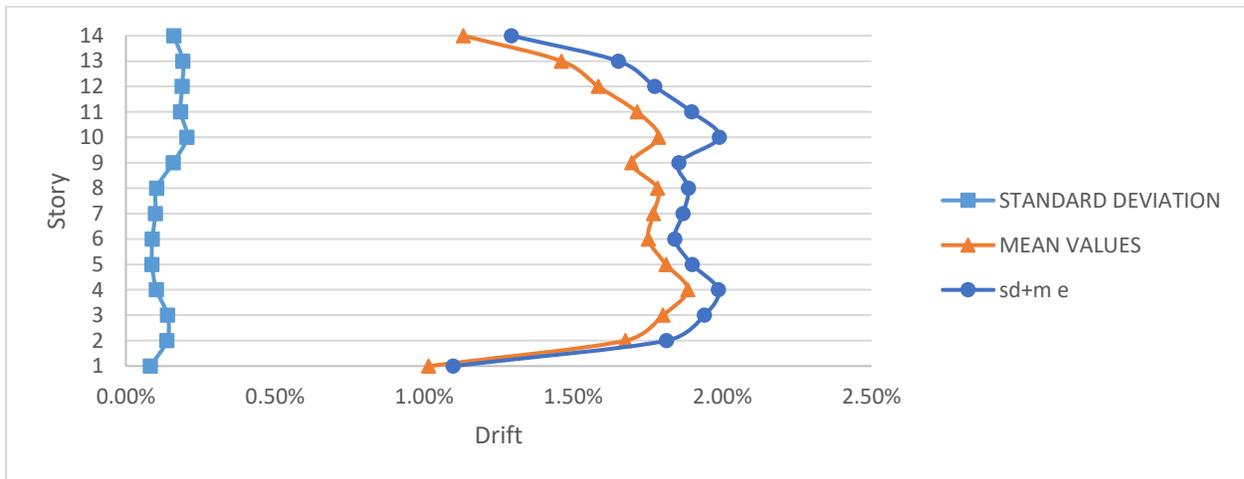
Figure 4-21 Standard deviation, mean values and sum for the Time History drift for ductile model (DUC)
