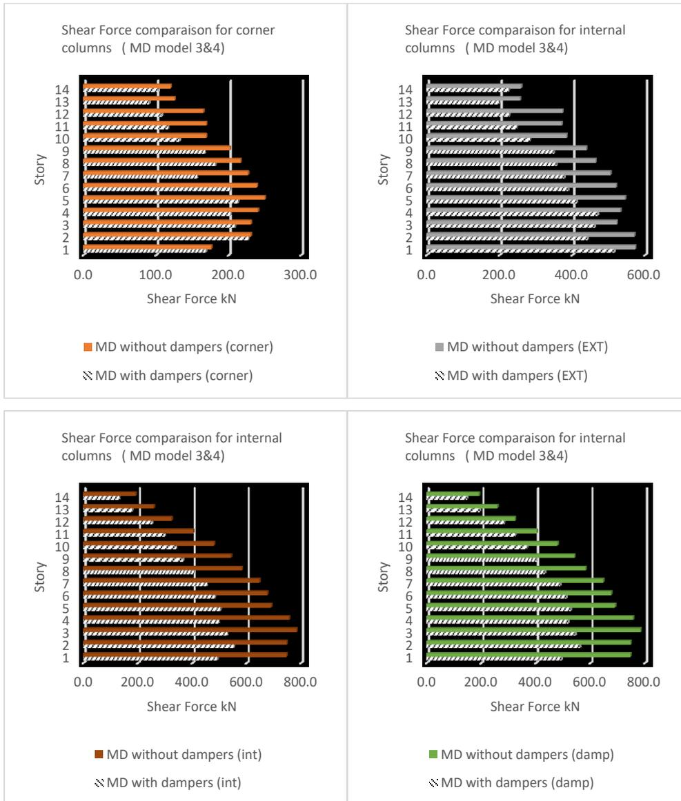
Figure 3-6 Shears Force columns comparisons between model (MD) & (MD-D): (a) between corner columns (b) between external columns (c) between internal columns (DUC) between internal columns connected to a dampers.
