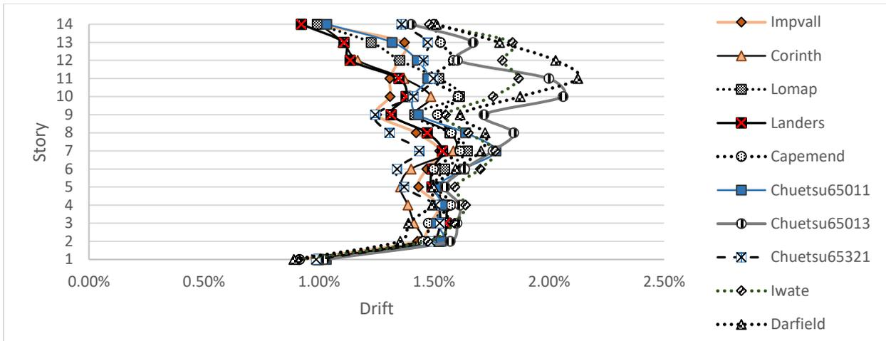
Figure 4-22 Time History drift for ductile model with dampers (DUC-D)
