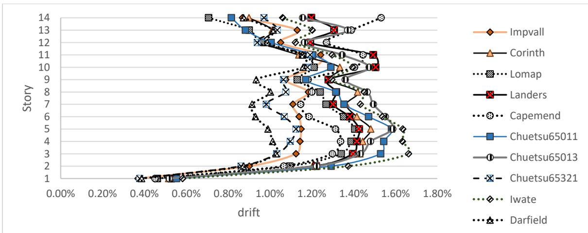
Figure 4-17 Time History drift for moderately- ductile model with dampers (MD-D)
