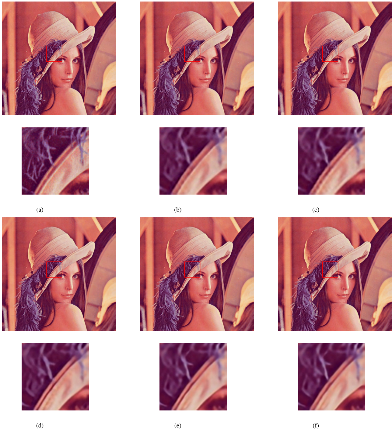
FIGURE 2. Visual comparison between CompNet and the other state-of-the-art methods when applied to the Lena image with upscaling factor 3. (a) Ground truth. (b) A+ (PSNR = 33.55, SSIM = 0.8862). (c) SRCNN (PSNR = 33.70, SSIM = 0.8878). (d) CSCN (PSNR = 33.70, SSIM = 0.8879). (e) VDSR (PSNR = 33.99, SSIM = 0.8915). (f) CompNet (PSNR = 34.02, SSIM = 0.8920).
