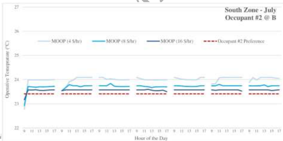
Fig. 7: The influence of productivity per hour ($/h) on the thermal comfort of occupants – The warm season analysis
