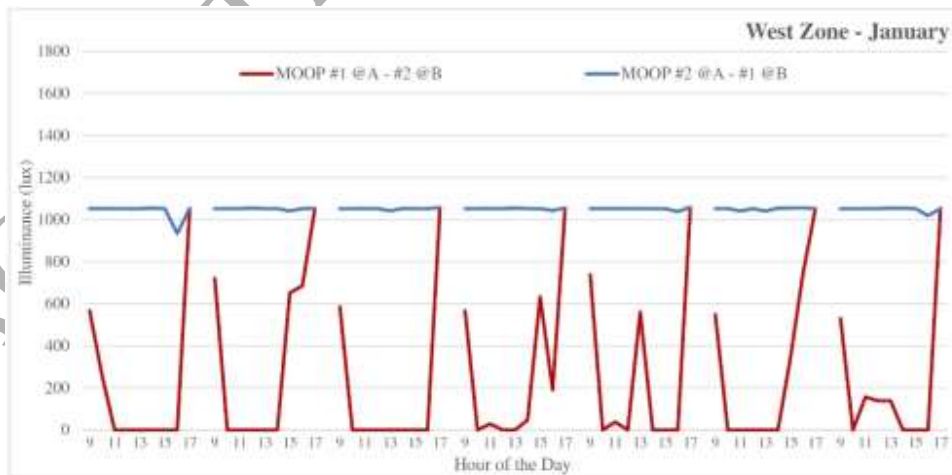
Fig. 19: Different occupancy scenarios and the level of artificial lighting (lux) – The cold season analysis
