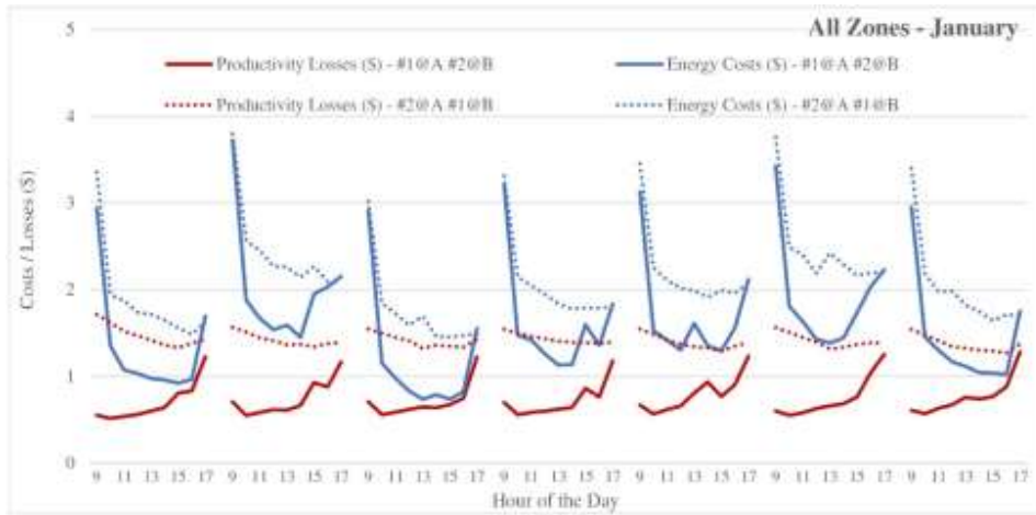
Fig. 21: The importance of occupants' positions for the productivity losses ($) and energy costs ($) - The cold season analysis
