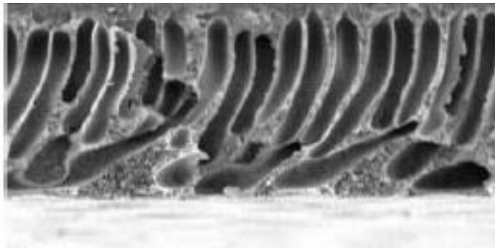
Figure 2. 3 Thin film composite structure of RO membrane with TFC structure 25 .
