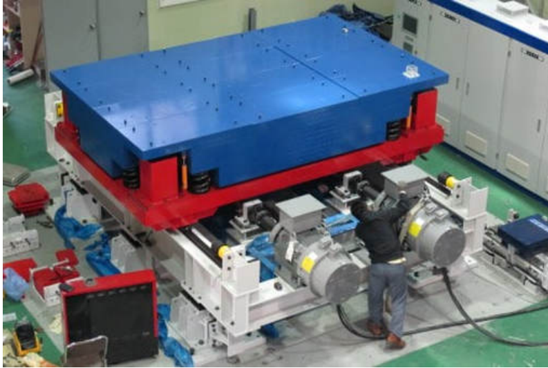
Figure 2-19 : Technomart Hybrid Mass Damper with 50 ton moving mass at TESolution structural lab-South Korea (TESolution www.tesolution.com , June 2018)
