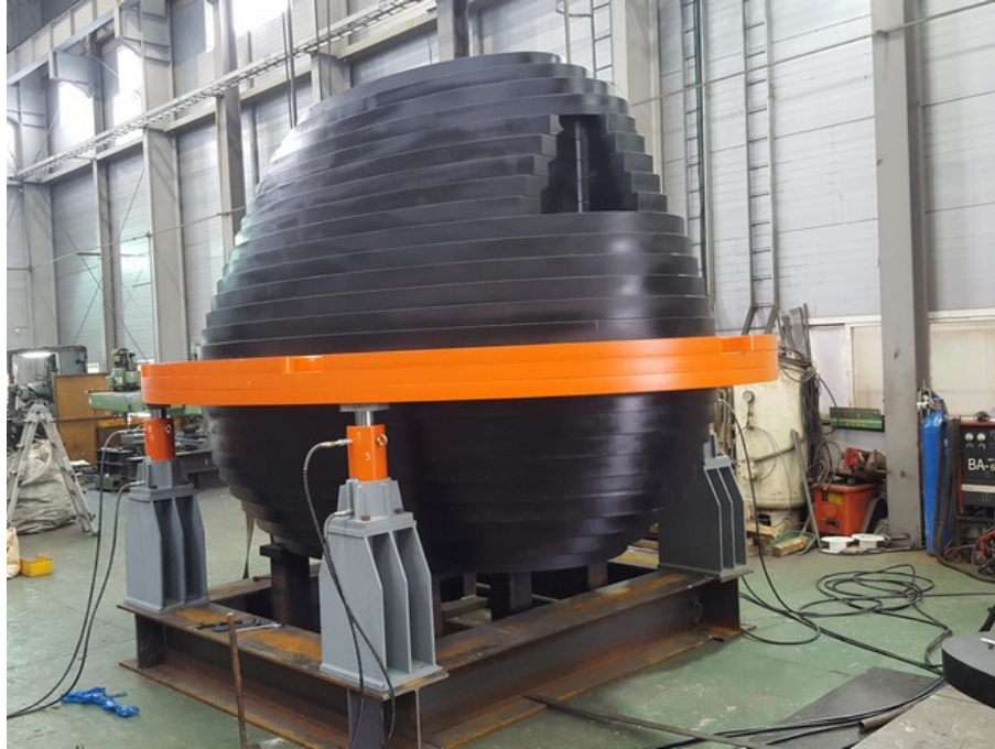
Figure 2-6: A pendulum type 150 ton TMD designed and manufactured by TESolution company for a residential tower -Taichung- South Korea (TESolution www.tesolution.com , June 2018)
