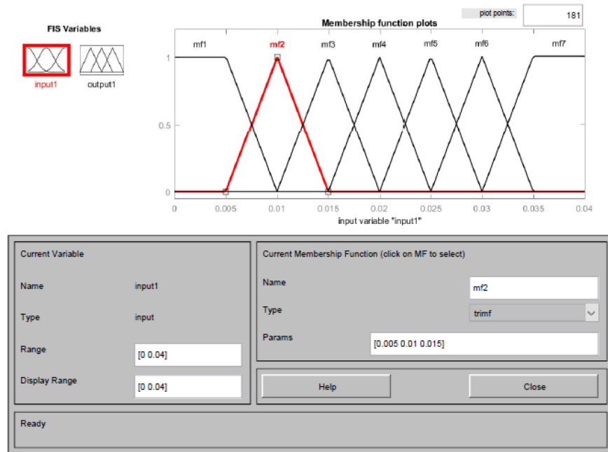
Figure 4-4: The defined input membership functions (Displacement) in MATLAB software
