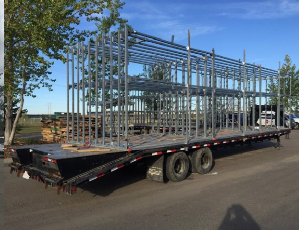
Figure 4.20: Special steel frames on trailer for panel transportation
