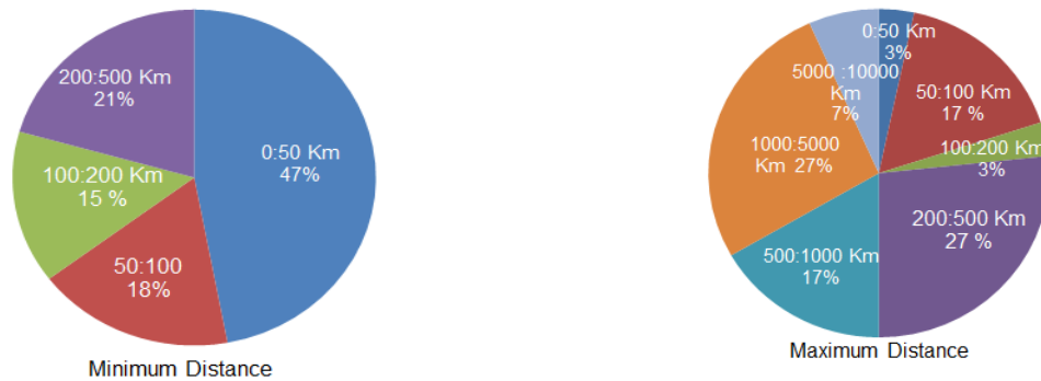
Figure I.15 : Common distance between manufacturing facility and project construction site for modular projects
