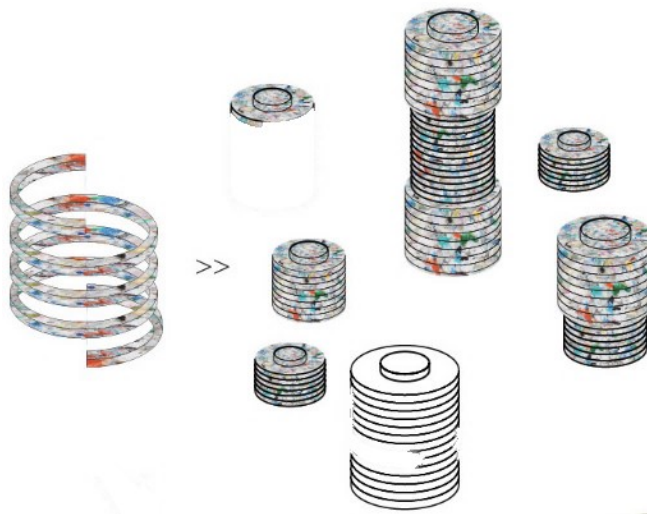
Figure 28: Proposed elements. These are made of layers of recycled melted plastic that allows multiple configurations depending on the needs.
