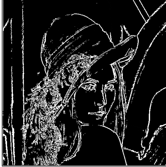
Figure 22: Image after Hysteresis Thresholding
