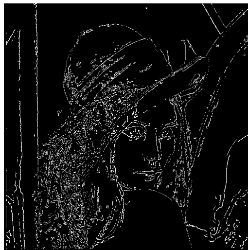
Figure 23: Final image after Canny Edge Detection
