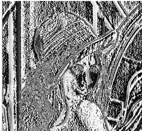
Figure 17: Image gradient along the X direction
