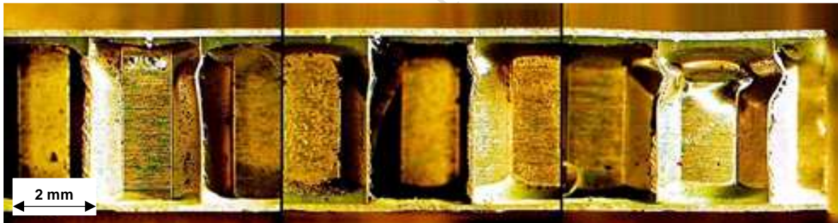
Figure 14: Core damage in experimental coupon for face sheet dent depths of 0.04 mm (left), 0.10 mm (middle), and 0.29 mm (right)
