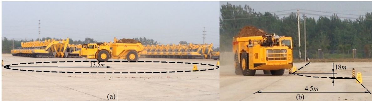
Figure 3.6: Test courses: (a) steady-turning maneuver; (b) path-change maneuver [131]
