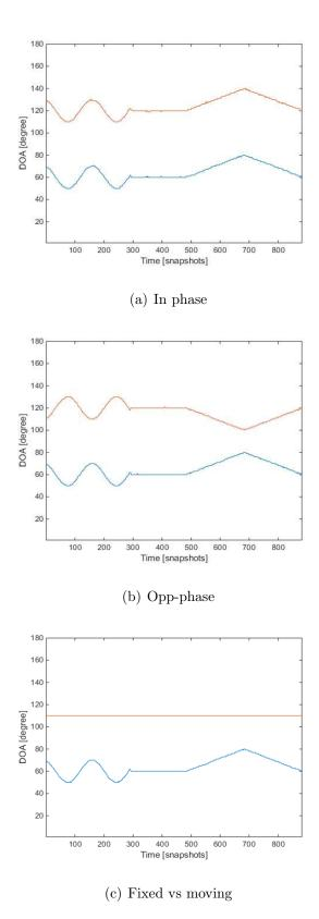
Figure 5.31: Trajectories of two source signals using MBS MVDR A-LASSO DOA estimation technique, 10 snapshots, SNR = 10 dB, type II fluctuating sources.
