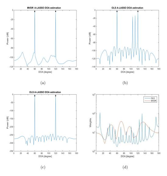
Figure 3.13: DOA estimation using A-LASSO algorithms, for two source signals at DOAs  $60^{\circ}$  and  $120^{\circ}$ , 10 snapshots, SNR = 0 dB. (a) MVDR A-LASSO after the first iteration; (b) OLS A-LASSO after the first iteration; (c) OLS A-LASSO after five iterations; and (d) initial weights of the two algorithms.
