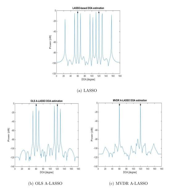
Figure 3.5: Performance of LASSO, OLS A-LASSO and MVDR A-LASSO, for two source signals at DOAs 60° and 120°, 10 snapshots, SNR = 0 dB and one iteration. (a) LASSO; (b) OLS A-LASSO; and (c) MVDR A-LASSO.
