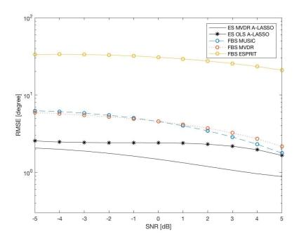
Figure 5.12: Performance comparison of the different algorithms as SNR is varied using BS MVDR, BS MUSIC, BS ESPRIT, ES OLS A-LASSO (single iteration) and ES MVDR A-LASSO (single iteration).
