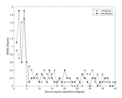
Figure 3.21: RMSE for each of the signals as a function of the separation between two sources, SNR = 10 dB, 10 snapshots and one iteration of MVDR A-LASSO.
