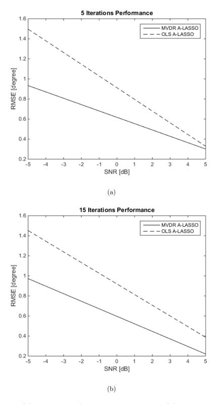
Figure 3.14: DOA estimation of two source signals at DOAs  $60^{\circ}$  and  $120^{\circ}$ , and 10 snapshots (a) after five iterations and (b) after 15 iterations, using the A-LASSO algorithms.
