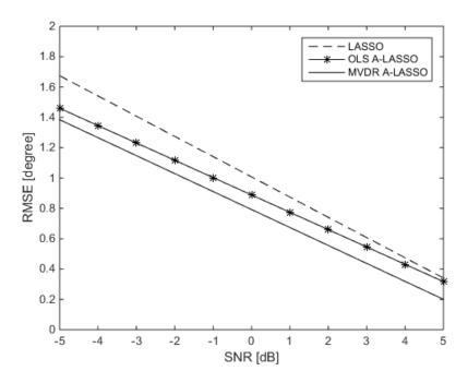
Figure 3.6: Performance of the three LASSO algorithms versus SNR, for two source signals at DOAs 60° and 120°, 10 snapshots and after one iteration of the MVDR A-LASSO and OLS A-LASSO algorithms.
