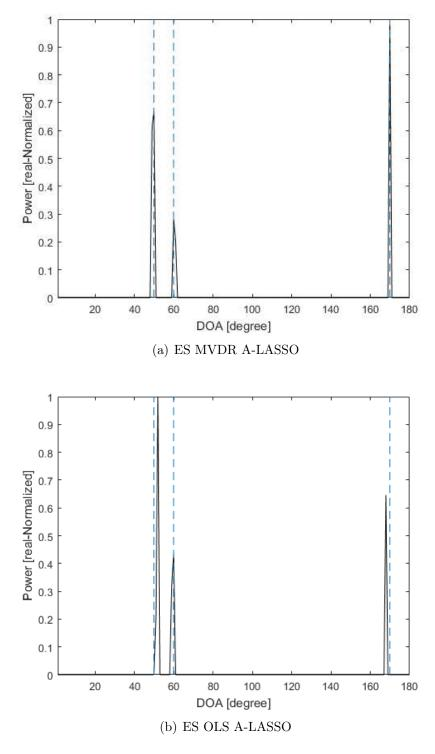
Figure 5.9: DOA estimation for 3 source signals with DOAs  $50^{\circ}$ ,  $60^{\circ}$  and  $170^{\circ}$ , uncorrelated sources, single snapshot, single iteration and AWGN with SNR = 0 dB, using (a) ES MVDR A-LASSO and (b) ES OLS A-LASSO.
