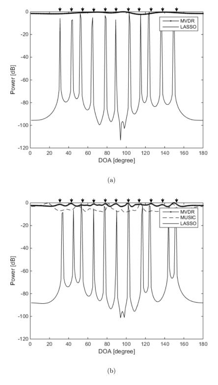
Figure 3.9: DOA estimation when the number of sources is more than the number of sensors: (a) Classical LASSO and MVDR using a six-element array; (b) Classical LASSO, MVDR and MUSIC using a 23-element array.
