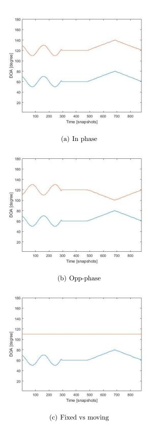
Figure 5.29: Trajectories of two source signals using MBS MVDR A-LASSO DOA estimation technique, 10 snapshots,  $\rm SNR=10~dB$ , non-fluctuating sources.
