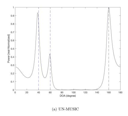
Figure 4.5: DOA estimation for 3 source signals with DOAs  $40^\circ,60^\circ$  and  $160^\circ,$  uncorrelated sources, 10 snapshots, and pink noise and AWGN with SNR = 0 dB, using UN-MUSIC.
