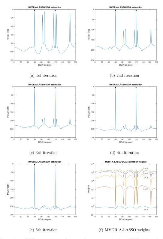
Figure 3.16: DOA estimation in the case of two source signals at DOAs 60° and 120°, SNR = -10 dB, 150 snapshots, using the MVDR A-LASSO algorithm. (a–e), after one to five iterations; and (f) MVDR A-LASSO weights as the number of iterations k varies.
