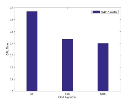
Figure 5.36: CPU time as a measure for the computational complexity of the proposed MVDR A-LASSO-based DOA estimation techniques.
