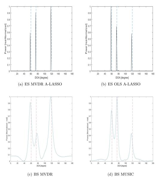
Figure 5.4: DOA estimation of 3 sources using a ULA containing 7 elements, SNR = 0 dB, using (a) ES MVDR A-LASSO, (b) ES OLS A-LASSO, (c) BS MVDR, and (d) BS MUSIC.
