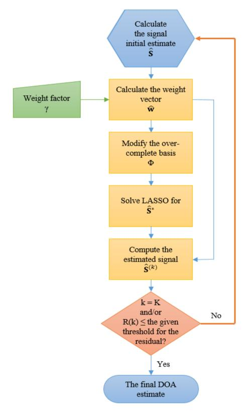
Figure 3.1: A flowchart of the algorithm for A-LASSO-based DOA estimation.
