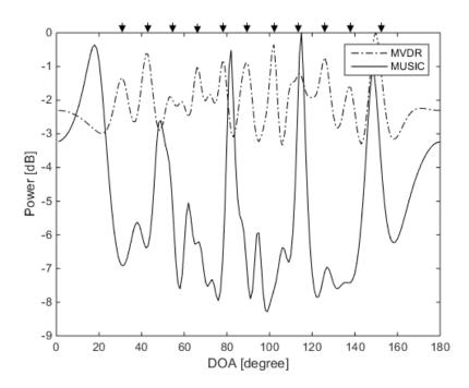
Figure 3.10: DOA estimation when the number of sources is more than the number of sensors: MVDR and MUSIC using a 23-element array.
