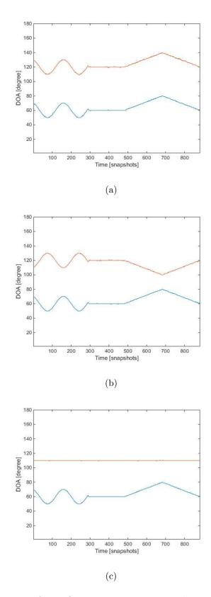
Figure 3.28: Trajectory of two fluctuating source signals using MVDR A-LASSO,  $\rm SNR=10~dB.$  (a,b, and c) Swerling-II, 10 snapshots.
