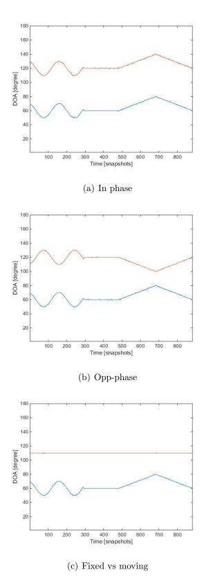
Figure 5.26: Trajectories of two source signals using FBS MVDR A-LASSO DOA estimation technique, 10 snapshots, SNR = 10 dB, type II fluctuating sources.
