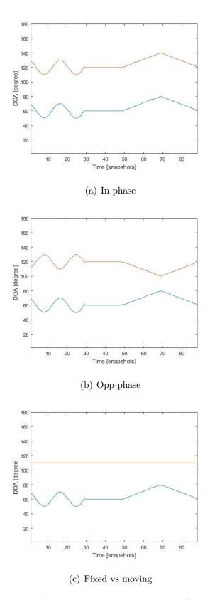
Figure 5.27: Trajectories of two source signals using FBS MVDR A-LASSO DOA estimation technique, 100 snapshots,  $\rm SNR=10$  dB, type III fluctuating sources.
