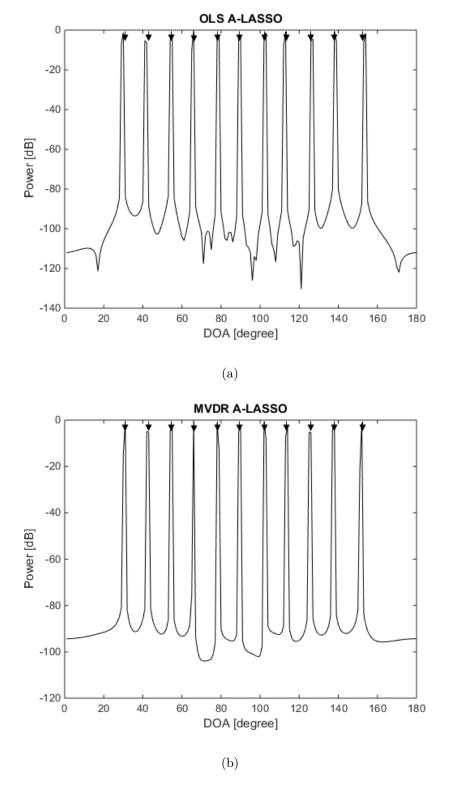
Figure 3.8: DOA estimation when the number of sources is more than the number of sensors: (a) After one iteration of OLS A-LASSO and (b) After one iteration of MVDR A-LASSO.
