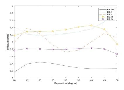
Figure 3.23: RMSE for two sources as a function of separation between the DOAs of the sources, SNR = 0 dB, 10 snapshots using MVDR A-LASSO.
