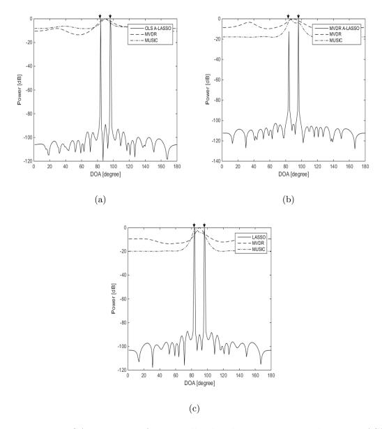
Figure 3.11: DOA estimation for spatially-closed two-source signals using LASSO algorithms, for two source signals at DOAs 85° and 95°, 10 snapshots, SNR = 15 dB and one iteration of the MVDR A-LASSO and OLS A-LASSO algorithms. (a) OLS A-LASSO after the first iteration; (b) MVDR A-LASSO after the first iteration; and (c) the classical LASSO algorithm.
