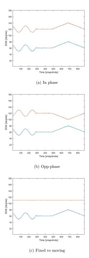
Figure 6.5: Simulink-based DOA estimation for non-fluctuating source signals, SNR = 0 dB, External Mode, using FBS MVDR A-LASSO.
