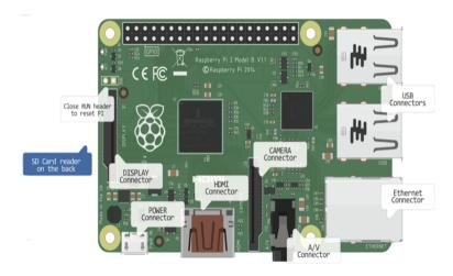
Figure 6.1: Top view of a Raspberry Pi 2 Model B.
