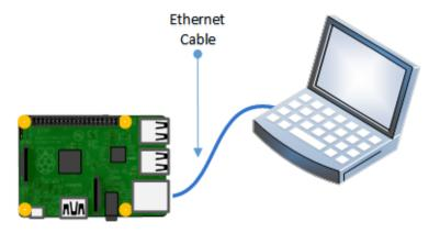
Figure 6.2: Direct connection between Raspberry Pi board and PC using Ethernet cable.
