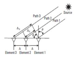
Figure 2.1: Simple Antenna Array Configuration [11]
