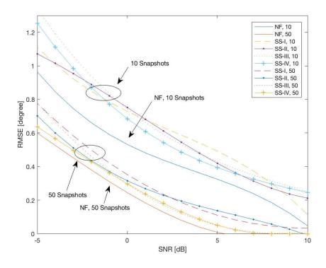
Figure 3.22: Performance of MVDR A-LASSO as SNR is varied, for two fluctuating source signals at DOAs 60° and 120°, using different Swerling source signals models.
