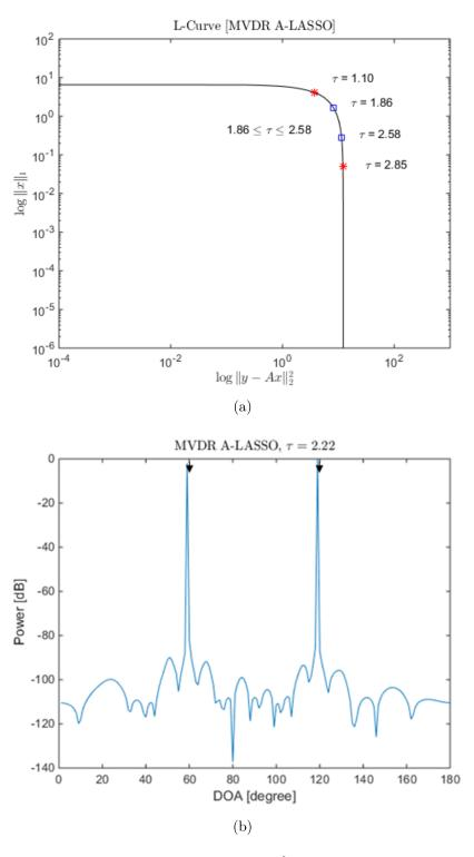
Figure 3.3: (a) The data residual  $\|\mathbf{y} - \Phi^* \bar{\mathbf{s}}\|_2^2$  versus the solution  $\ell_1$ -norm linear scale on a log-log scale (L-curve); (b) DOA estimation for two source signals;  $\tau$  was selected using L-curve, in the MVDR A-LASSO problem (SNR = 0 dB).
