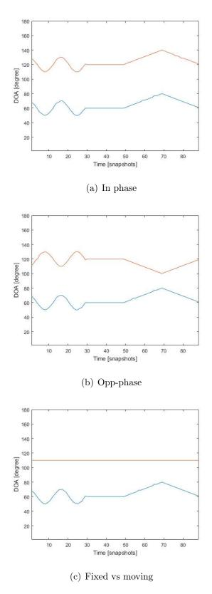
Figure 5.25: Trajectories of two source signals using FBS MVDR A-LASSO DOA estimation technique, 100 snapshots, SNR = 10 dB, type I fluctuating sources.
