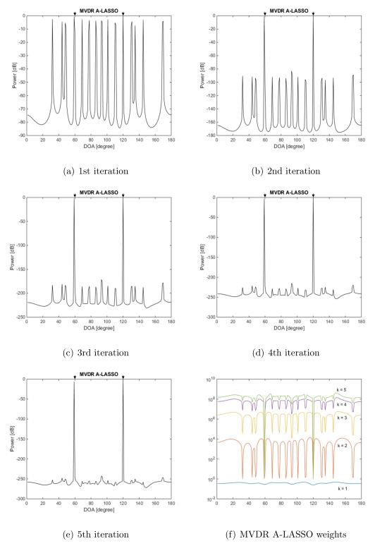
Figure 3.17: DOA estimation, two source signals at DOAs  $60^{\circ}$  and  $120^{\circ}$ , SNR = -15 dB, 200 snapshots, using the MVDR A-LASSOalgorithm. (a–e) after one to five iterations; and (f) MVDR A-LASSO weights as the number of iterations k varies.
