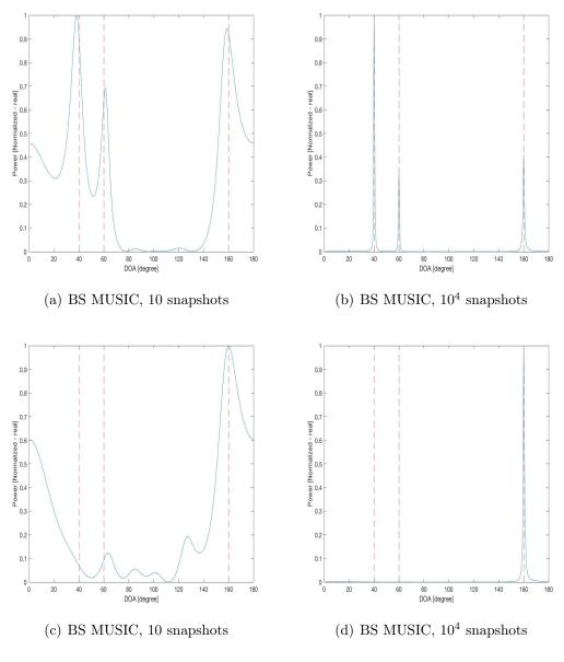
Figure 5.8: DOA estimation for 3 source signals with DOAs  $40^{\circ}$ ,  $60^{\circ}$  and  $160^{\circ}$ , SNR = 0 dB, using BS MUSIC. (a) and (b) uncorrelated sources, (c) and (d) two of the sources being correlated.
