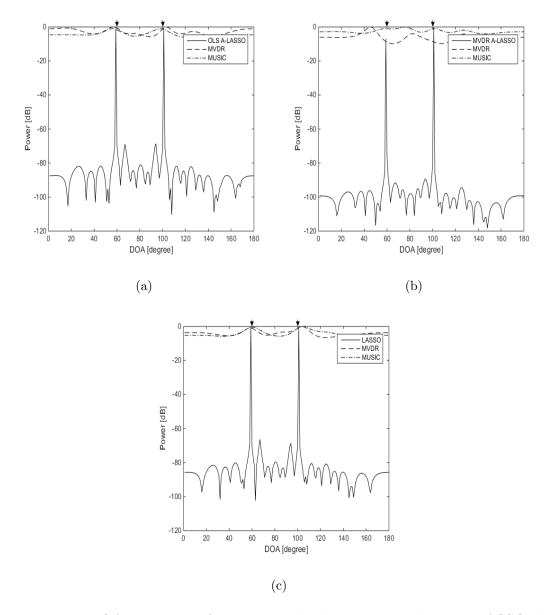
Figure 3.12: DOA estimation for two correlated source signals using LASSO algorithms, for two source signals at DOAs 60° and 100°, 10 snapshots, SNR = 15 dB and one iteration of the MVDR A-LASSO and OLS A-LASSO algorithms. (a) OLS A-LASSO after the first iteration; (b) MVDR A-LASSO after the first iteration; and (c) the classical LASSO algorithm.
