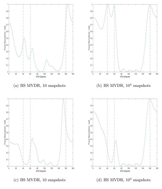
Figure 5.7: DOA estimation for 3 source signals with DOAs  $40^{\circ}$ ,  $60^{\circ}$  and  $160^{\circ}$ , SNR = 0 dB, using BS MVDR. (a)and (b) uncorrelated sources, (c) and (d) two of the sources being correlated.
