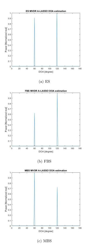
Figure 6.3: Simulink-based DOA estimation for two source signals at  $60^{\circ}$  and  $120^{\circ}$ , 10 snapshots, SNR = 0 dB, External Mode, using MVDR A-LASSO (a) ES, (b) FBS, and (c) MBS.
