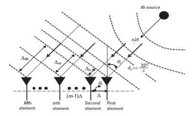
Figure 2.2: Data model for DOA using ULA [11]
