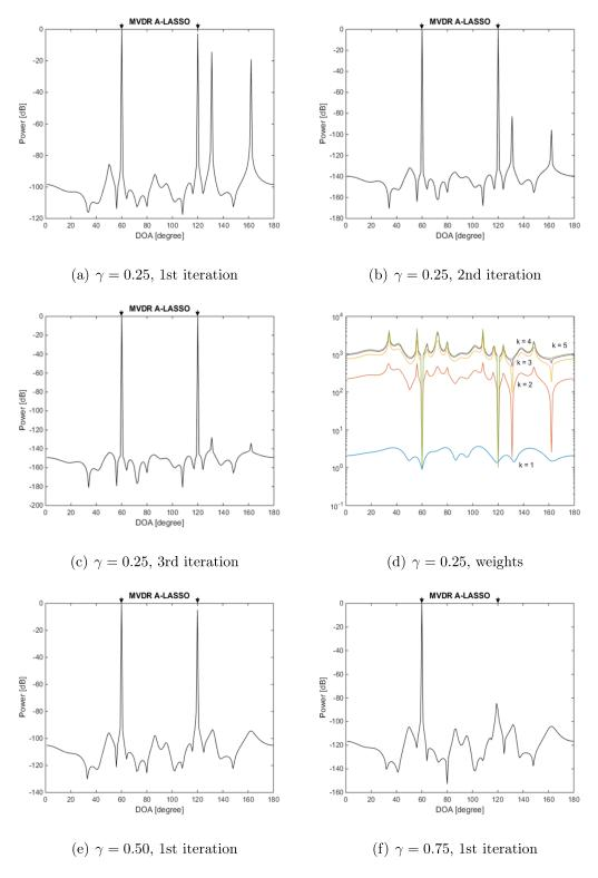
Figure 3.20: DOA estimation of two source signals at DOAs 60° and 120°, 50 snapshot, SNR = -5 dB, using the MVDR A-LASSO algorithm, (a)–(d)  $\gamma = 0.25$ ; (e)  $\gamma = 0.50$ ; and (f)  $\gamma = 0.75$ .
