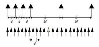
Figure 3.4: The proposed sparse (**upper**) and the virtual co-array (**lower**).
