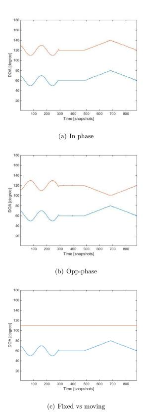
Figure 5.33: Trajectories of two source signals using MBS MVDR A-LASSO DOA estimation technique, 10 snapshots, SNR = 10 dB, type IV fluctuating sources.
