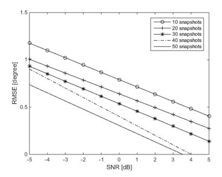
Figure 3.18: MVDR A-LASSO DOA estimation performance versus the number of snapshots, two source signals with DOAs  $60^{\circ}$  and  $120^{\circ}$ ,  $\gamma = 0.5$ .
