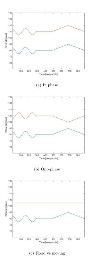
Figure 5.28: Trajectories of two source signals using FBS MVDR A-LASSO DOA estimation technique, 10 snapshots, SNR=10 dB, type IV fluctuating sources.
