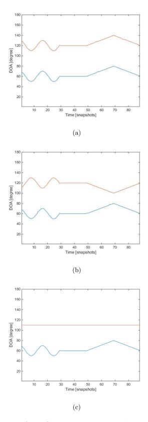
Figure 3.29: Trajectory of two fluctuating source signals using MVDR A-LASSO,  $\rm SNR=10~dB.$  (a,b, and c) Swerling-III, 100 snapshots.
