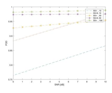
Figure 5.22: Probability of detection of different Swerling source signals, two source signals with DOA of  $60^{\circ}$  and  $120^{\circ}$ , using MBS algorithm.
