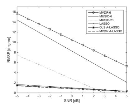
Figure 3.7: Performance of the LASSO algorithms as SNR is varied in comparison with that of MVDR and MUSIC algorithms, for two source signals at DOAs 60° and 120°, 10 snapshots and after one iteration of the MVDR A-LASSO and OLS A-LASSO algorithms.
