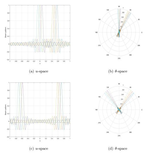
Figure 5.13: Beam pattern, multiple beam,  $M=31,~N_{bs,1}=N_{bs,2}=3,$  (a)  $\theta_{c1}=60^\circ,\theta_{c2}=90^\circ$  and (b)  $\theta_{c1}=50^\circ,\theta_{c2}=130^\circ.$
