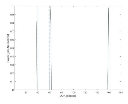
Figure 4.6: DOA estimation for 3 source signals with DOAs  $40^{\circ}$ ,  $60^{\circ}$  and  $160^{\circ}$ , where the first 2 source signals are fully correlated, 10 snapshots, and pink noise and AWGN with SNR = 0 dB, using (a) GCD MVDR A-LASSO and (b) GCD OLS A-LASSO.
