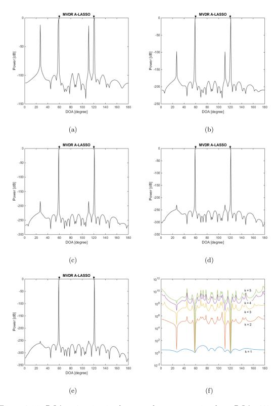
Figure 3.15: DOA estimation in the case of two source signals at DOAs 60° and 120°, SNR = -5 dB, 50 snapshots using MVDR A-LASSO algorithm. (a–e) after 1 – 5 iterations; and (f) MVDR A-LASSO weights as the number of iterations k varies.
