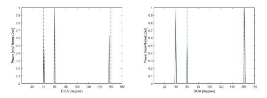
(a) FBS MVDR A-LASSO, single snapshot, (b) FBS MVDR A-LASSO, single snapshot, non-coherent coherent
