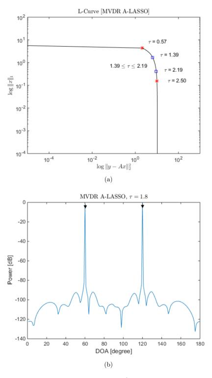
Figure 3.2: (a) The data residual  $\|\mathbf{y} - \Phi^*\bar{\mathbf{s}}\|_2^2$  versus the solution  $\ell_1$ -norm linear scale on a log-log scale (L-curve); (b) DOA estimation for two source signals;  $\tau$  was selected using L-curve, in the MVDR A-LASSO problem (SNR = 10 dB).
