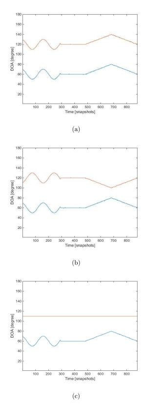
Figure 3.30: Trajectory of two fluctuating source signals using MVDR A-LASSO, SNR=10~dB. (a,b, and c) Swerling-IV, 10 snapshots.
