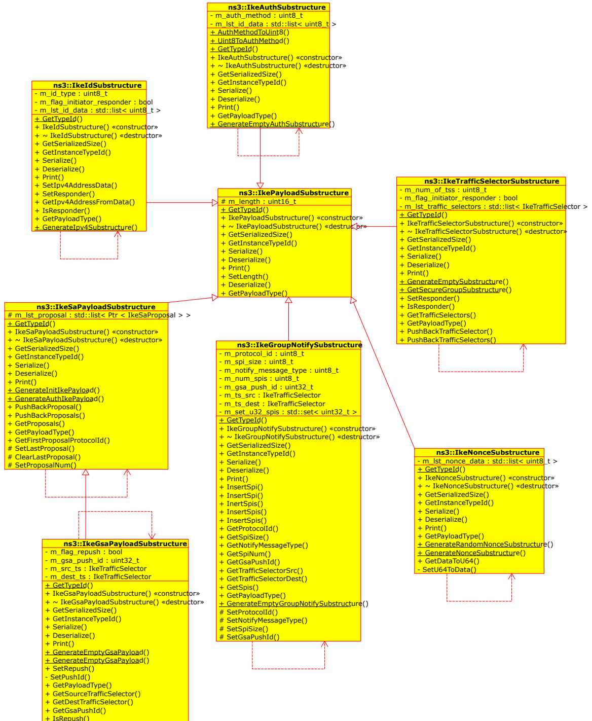
Figure A.13: The Class Diagrams of IKEv2 and GSAM Packet Payload Substructures Implementation
