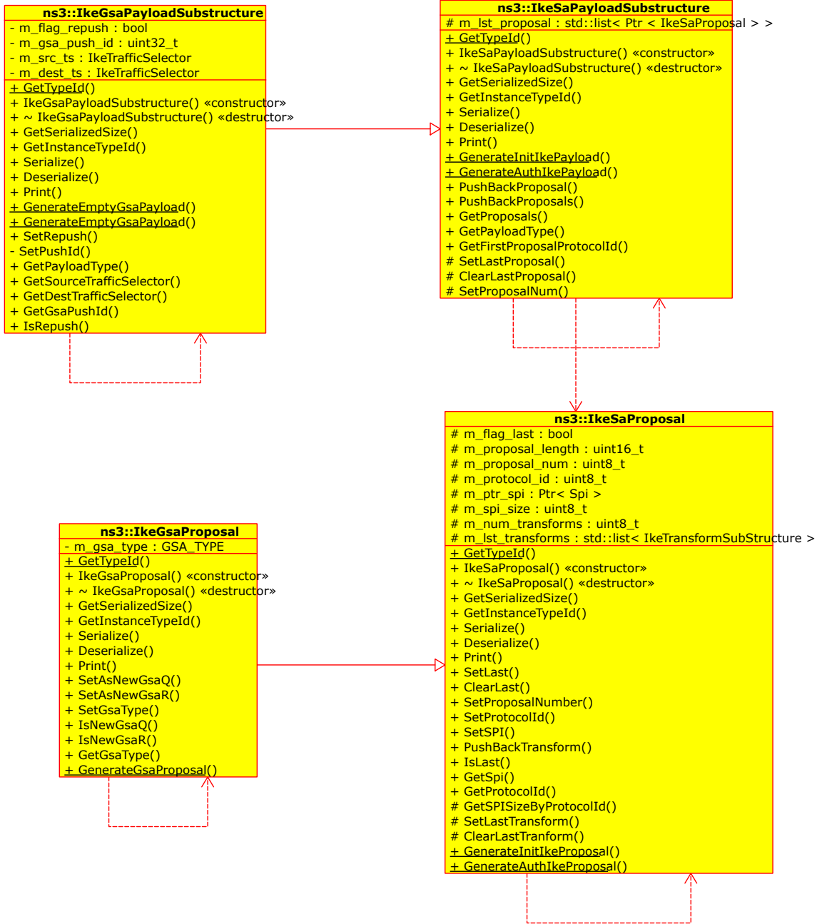
Figure A.14: The Class Diagrams of SA and GSA Payload Substructures Implementation
