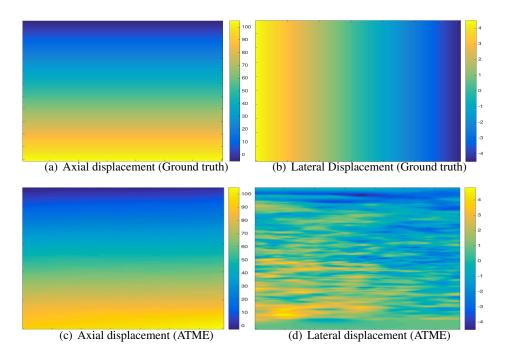
Figure 3.2: Field II and finite element simulation results. (a) and (b) show the axial and lateral ground truth displacement images of the simulation experiment. (c) and (d) are the corresponding axial and lateral displacement fields obtained from ATME.
