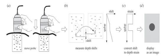
Figure 1.5: Quasi-static procedure. Image courtesy of (G. Treece et al., 2011)
