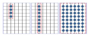
(a) NCC: displacement (b) DPAM: dis- (c) GLUE: displaceof windows are esti- placement of entire ment of all RF-lines are mated independently RF-line is estimated estimated simultaneindependently ously
