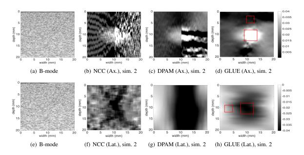
Figure 2.3: Field II and FEM simulation results. A vertical slippage exists in the motion field at the middle of the image. (a) is the first ultrasound image. (b) to (d) are the axial strain images. (e) is the second ultrasound image. (f) to (h) are the lateral strain images. Target and background windows used for CNR calculation of the GLUE results are shown in red. The SNR is calculated for the background window.
