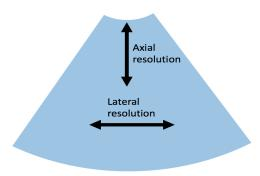
Figure 1.6: Axial and lateral resolution on the image produced by a sector scanner.
