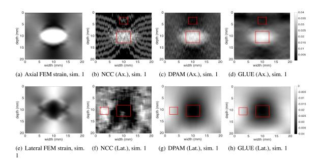
Figure 2.2: Field II and FEM simulation results. (a) is the axial ground truth strain. (b) to (d) show the axial strain images of the first simulation. (e) is the lateral ground truth strain. (f) to (h) show the lateral strain images of the first simulation. GLUE substantially outperforms NCC and DPAM in all results. Target and background windows used for CNR calculation are shown in red. The SNR is calculated for the background window.
