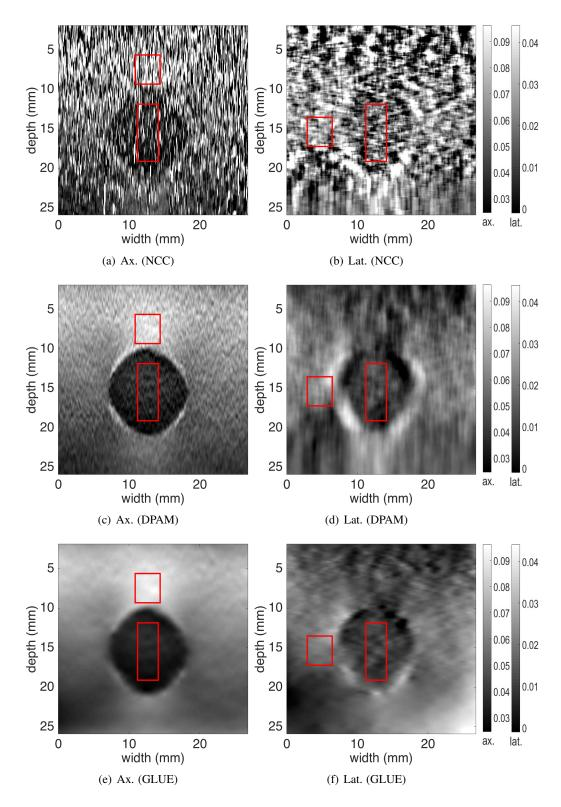
Figure 2.4: Results of the phantom experiment. Axial and lateral strain images as well as the target and background windows (in red) for calculation of SNR and CNR are shown (see Table 2.3 for results). The hard lesion is spherical and has a diameter of 1 cm. The axial and lateral strain scales are identical for NCC, DPAM and GLUE to ease comparison, and are shown in the right column.
