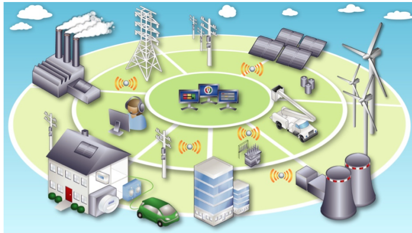
Figure 1.1: Smart Grid architecture. Sensors are deployed in different components of the grid such as generation, transmission, distribution, and consumption.
