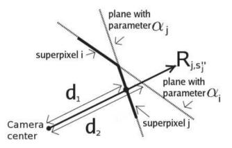
Figure 6: Make3D model for 3D reconstruction, here you can see two superpixels plane connected together, ray R is project on the planes and  $d_1 d_2$  are the distance, image is from Make3D work [SSN09a]
