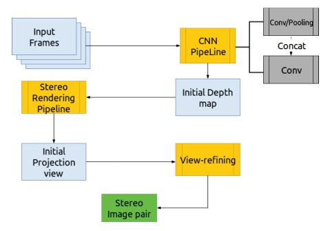
Figure 14: Pipeline with the neural network components
