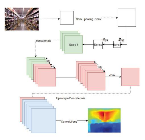
Figure 15: The diagram of the Convolutional Neural Network architecture we are using The first scale is represented in white, the second scale is in red and the last scale is blue .
