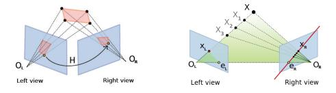
Figure 4: Homography Matrix vs Fundamental Matrix, homography matrix(left) map pixel to pixel and fundamental matrix(right) map pixels to a line. Images are from OpenMVG project
