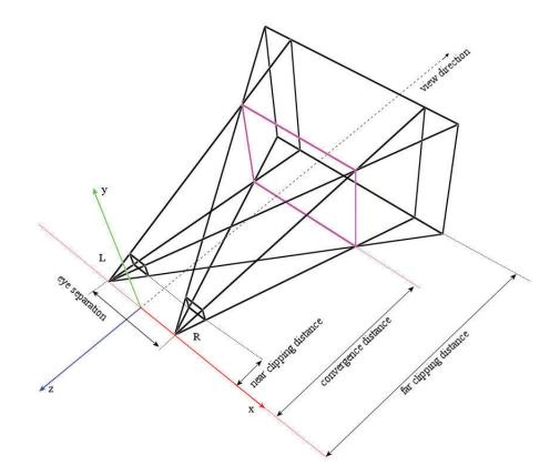
Figure 3: Stereo rendering through 3D geometries, image from [pag]
