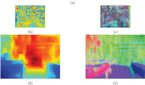
Figure 16: Output of the neural network: the image of the top row is the orignal RGB image; the two images on the second row are the low resolution depth and normal map; the last row are the finer resolution depth and normal map. Note that depth and normal map are post-processed with montage technique to be more colourful
