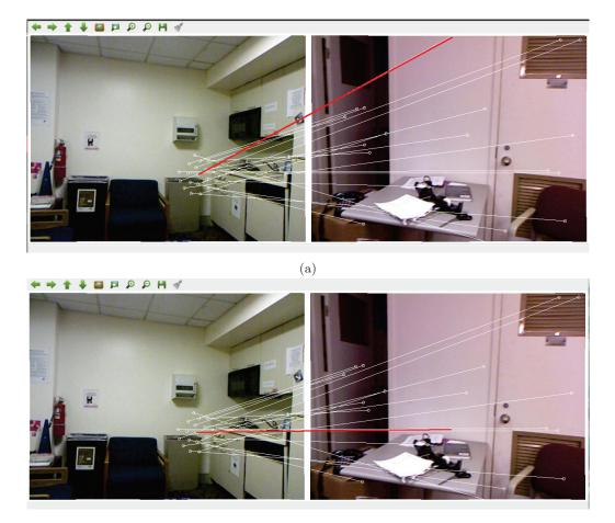
Figure 13: The optimizing process, image (a) is the matches before step, image (b) is the matches after optimizing step. Notice the **RED** line in (a), after moving the match, we can see that energy of geometry distances of matches decreases
