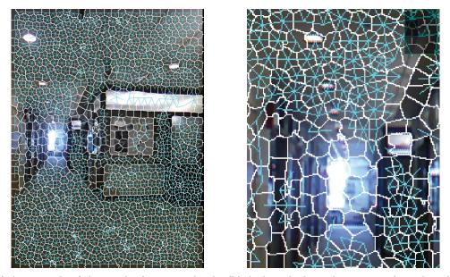
(a) An example of the graph of superpixels, the (b) A closer look on the superpixel graph under blue lines here indicate two superpixels are con- a smaller range of the the image nected
