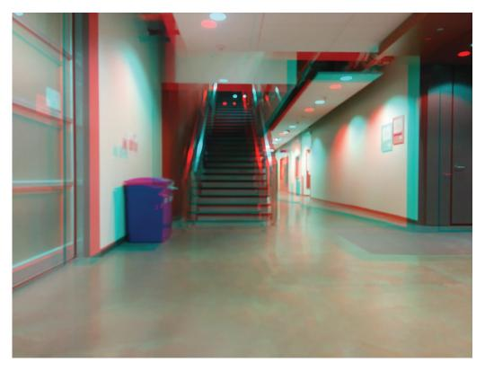
Figure 2: A sample Red-Cyan Anaglyph image taken at Concordia's EV building. To composite an anaglyph image, one can take one photo, then shift the camera along a direction for a short distance, then take another picture, and fuse them together
