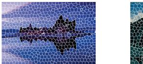
Figure 9: Superpixel representation, the image above is broken into non overlapped superpixels, a typical size image usually has a few hundred to one thousand superpixels.
