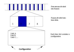
Figure 10: TDMA - Each frame achieves ConvergeCast
