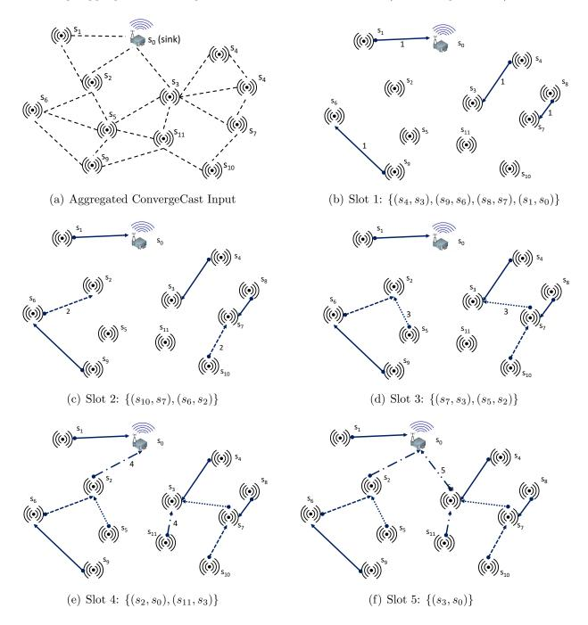
Figure 16: Aggregated ConvergeCast using 5 Configurations
