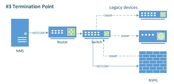
Figure 4.1: Possible proposed deployments for solution
