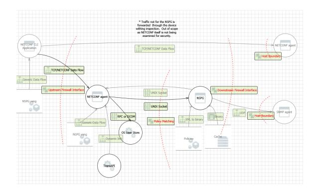
Figure 5.27: High-level threat model of the NSPG approach
