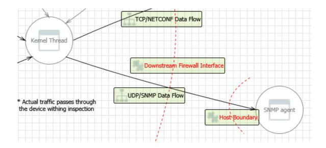
Figure 5.25: Dual-stack UDP/SNMP data flow figure (upstream)
