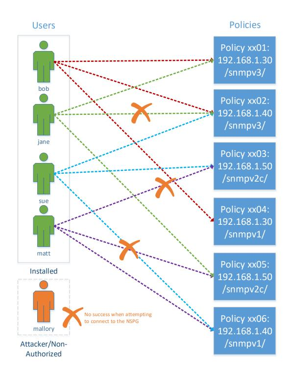
Figure 5.21: High-level diagram showing policy access successes and failures
