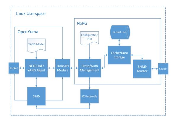
Figure 4.3: NSPG component block diagram (on the left is the upstream, right is downstream)
