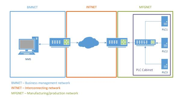
Figure 5.2: Simplifying the subset model network to demonstrate the path from NMS to legacy devices in a PLC cabinet
