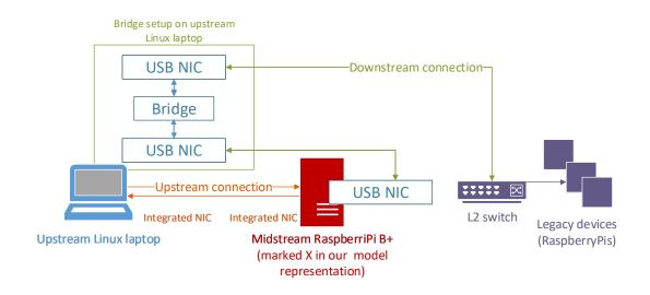
Figure 5.5: Test packet sniffing layout
