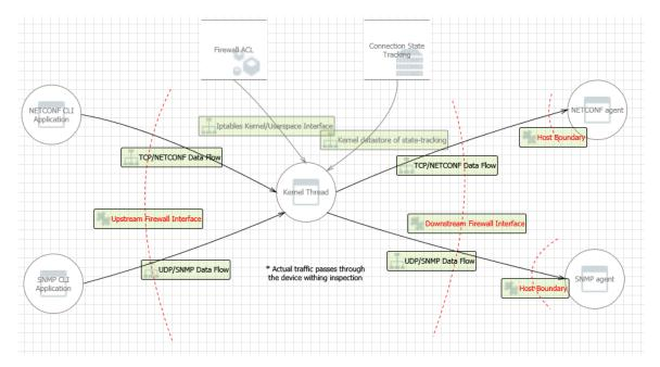
Figure 5.22: High-level threat model of the dual-stack approach
