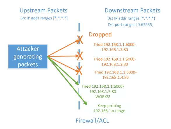
Figure 5.16: A simplified version of the ACL probing process used by attackers
