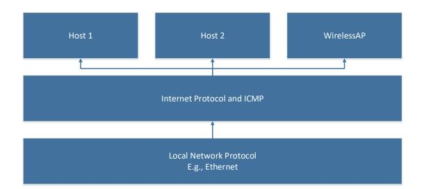
Figure 2.1: IP layer diagram
