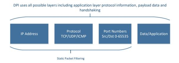
Figure 2.5: DPI vs static packet filtering diagram
