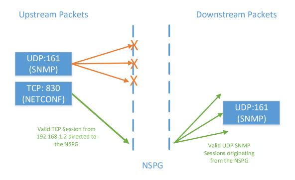
Figure 5.19: Simplified infographic of the NSPG and host dropping traffic, while only the NSPG can only generate SNMP traffic (on the downstream interface) based on policy configuration
