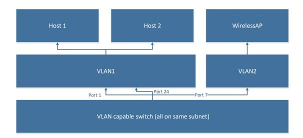
Figure 2.3: VLAN diagram
