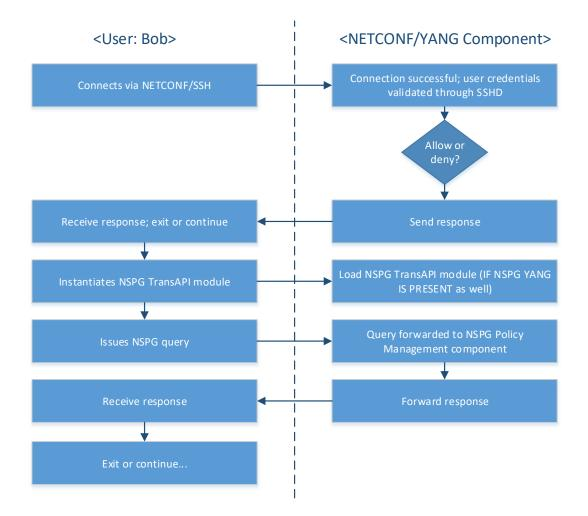
Figure 4.4: NSPG/YANG component swimlane diagram
