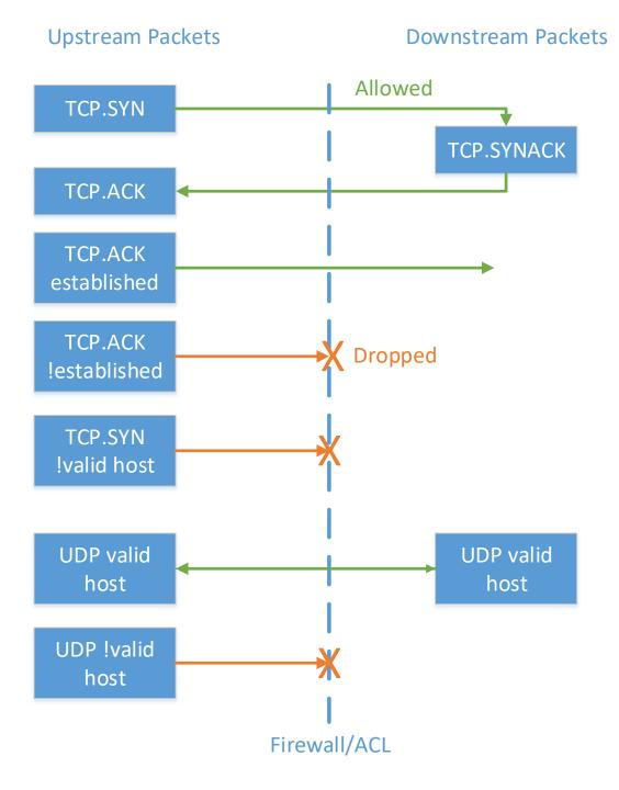
Figure 5.14: Infographic demonstrating normal packet ACL access/deny
