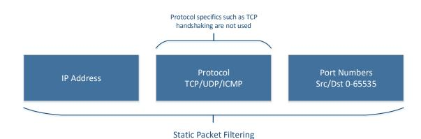
Figure 2.4: Static packet filtering diagram
