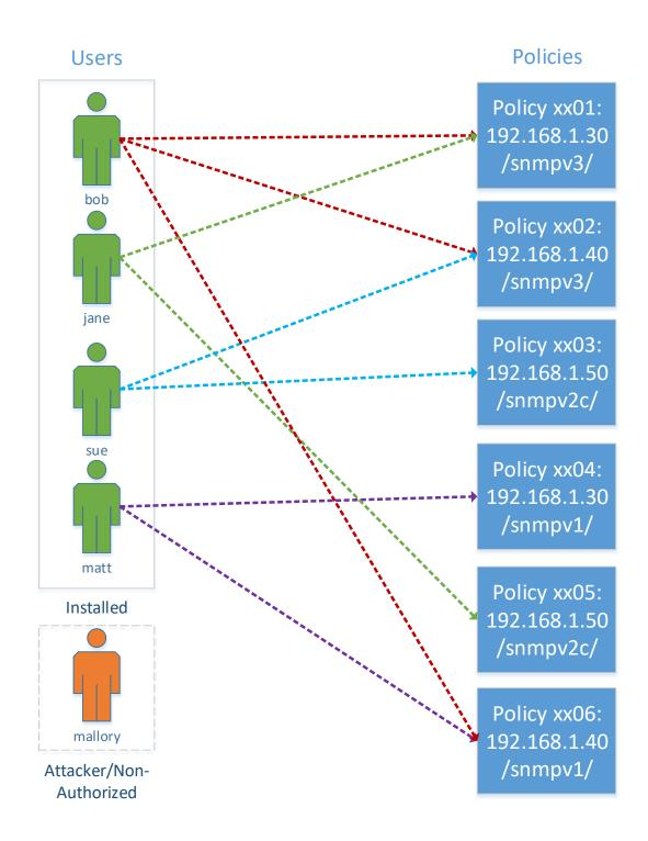
Figure 5.20: High-level diagram showing NSPG policy to user assignments
