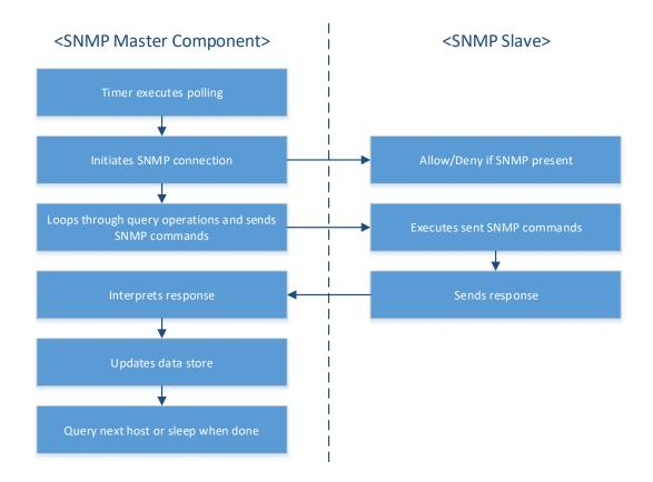
Figure 4.10: SNMP Master component swimlane diagram
