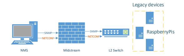
Figure 5.6: Dual-stack testing network topology
