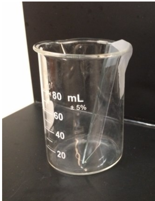
Figure 16 Picture of a beaker with a polymer slide kept at roughly 30 degrees, with scotch tape.
