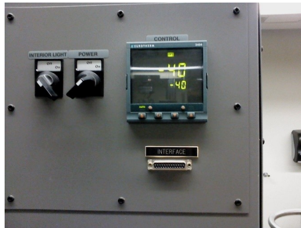
Figure 7.8 a) Environmental chamber enclosing the fixtures in the MTS machine, and attached to liquid nitrogen supply. b) 3-point bending fixtures holding the composite samples inside the environmental chamber and extensions attached to MTS machine and c) The controller of the environmental chamber showing that the set temperature of -40^{\circ}\text{C} has been reached
