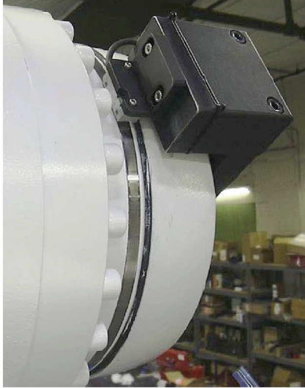
Figure 2.4: Secondary encoder installed on a KUKA robot [21]
