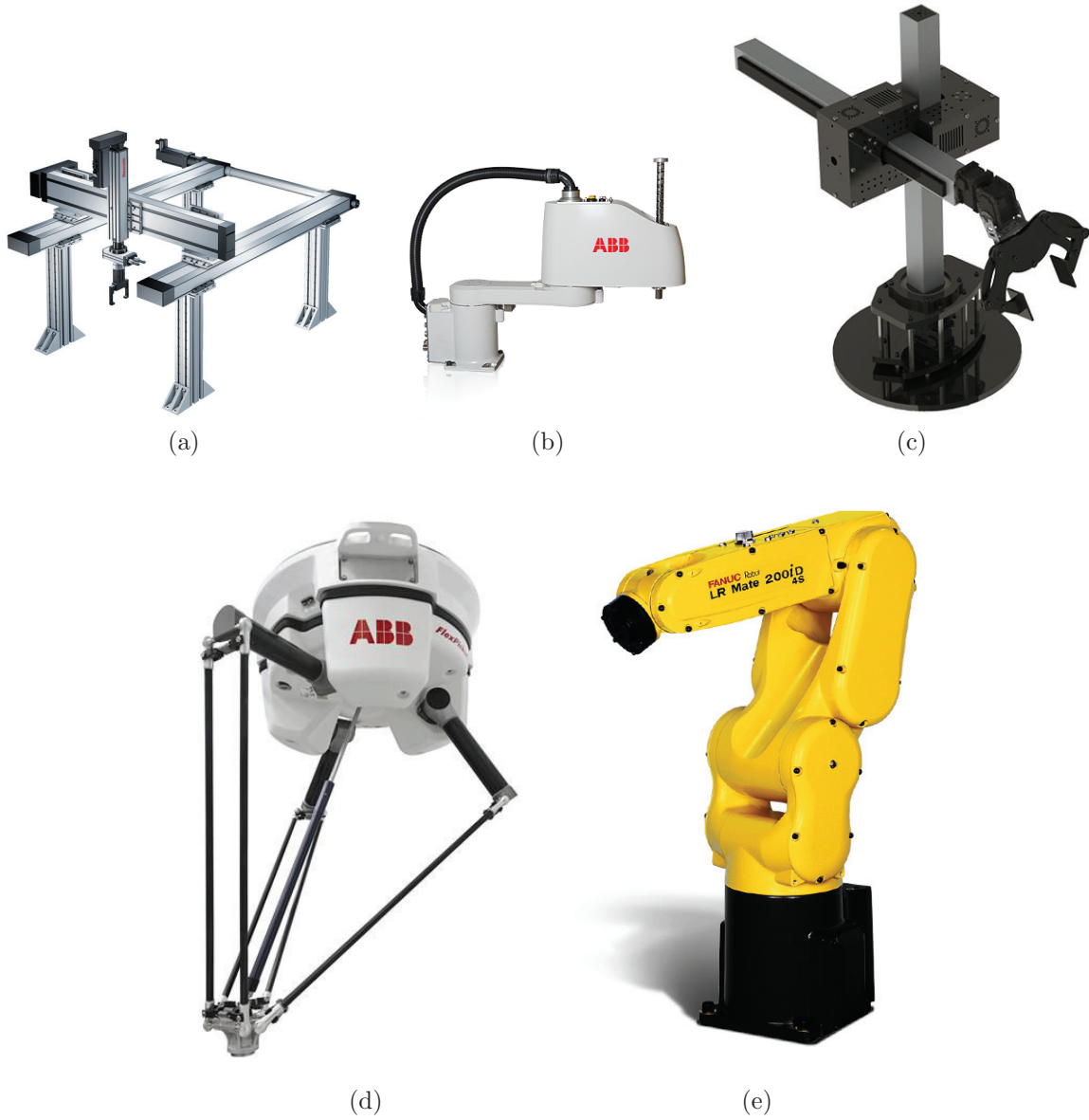
Figure 1.1: Different industrial robot types (a) Cartesian robot [8] (b) SCARA robot [9] (c) Cylindrical robot [10] (d) Delta robot [9] and (e) Serial robot [11]
