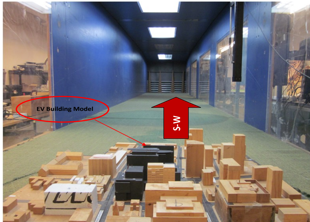
Fig. 2. 15: EV Building Model with the Surroundings under the Test in the Wind Tunnel (Direction of the Wind is South-West).
