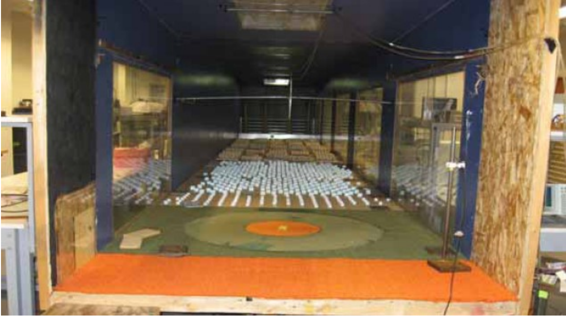
Figure 4 Front view section of the Boundary Layer Wind tunnel at Concordia University (from Stathopoulos et al. [6]).
