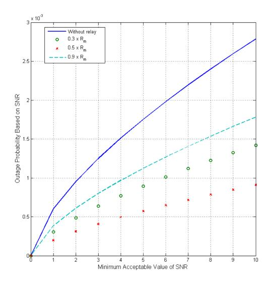
Figure 5.7: Outage probability based on SNR threshold for 6 relays located at 0.3  $\times$   $R_m,$  0.5  $\times$   $R_m$  and 0.9  $\times$   $R_m$
