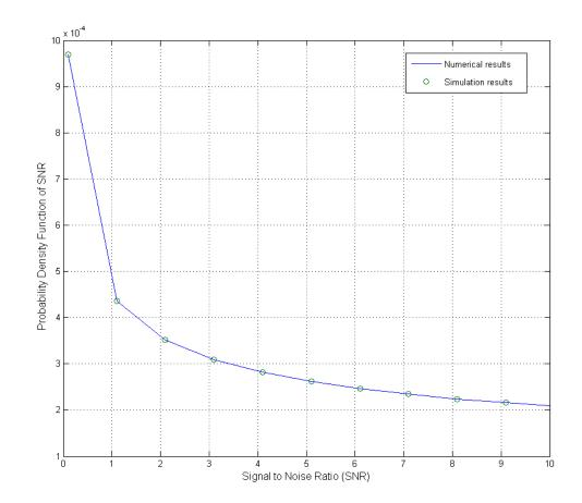
Figure 3.3: PDF of SNR in a circular cell
