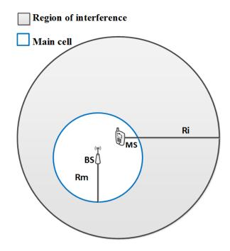
Figure 3.1: Main cell and region of interference for an arbitrary user MS
