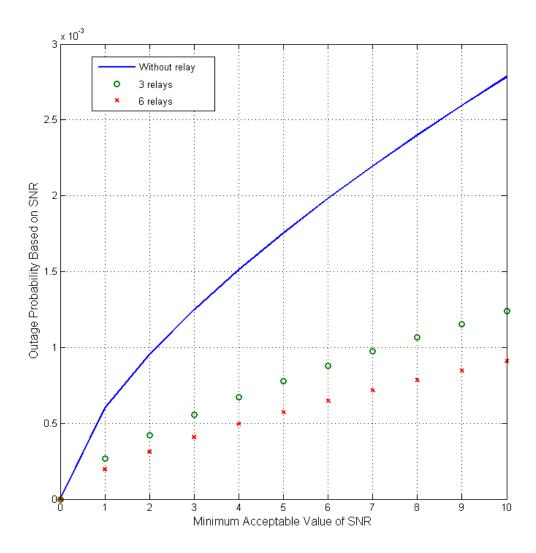
Figure 5.3: Outage probability based on SNR threshold for different number of relays located at 0.5  $\times$   $R_m$  from the BS
