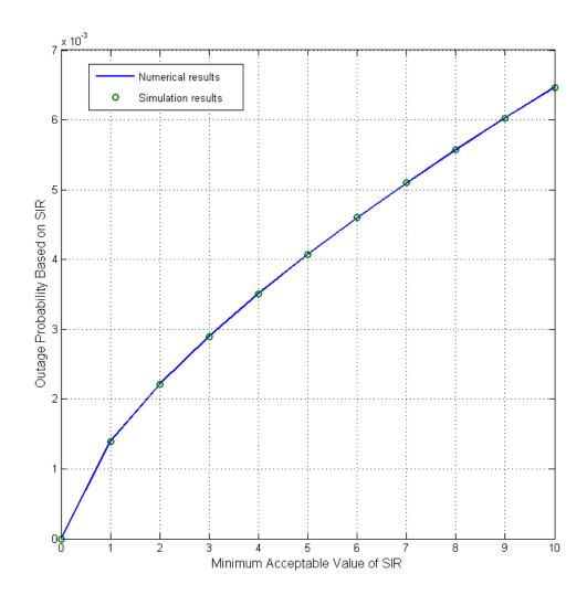
Figure 4.2: Outage probability based on SIR threshold in a circular cell
