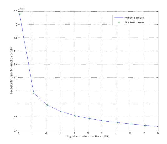
Figure 3.2: PDF of SIR in a circular cell
