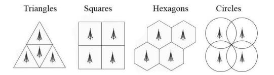
Figure 2.1: Circular cells versus cells with tessellating structures
