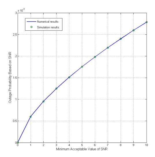
Figure 4.3: Outage probability based on SNR threshold in a circular cell
