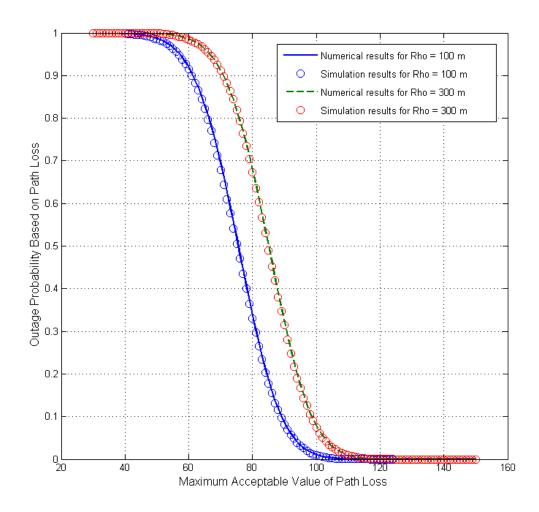
Figure A.1: Outage probability based on PL in a hexagonal cell for different cell sizes
