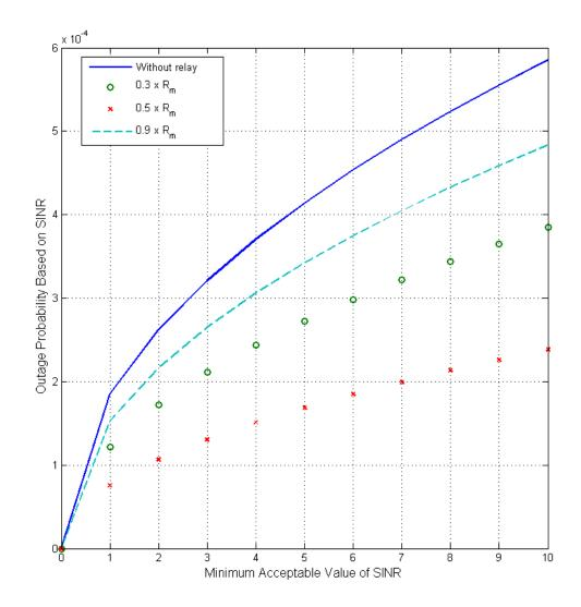
Figure 5.8: Outage probability based on SINR threshold for 6 relays located at 0.3  $\times$   $R_m,$  0.5  $\times$   $R_m$  and 0.9  $\times$   $R_m$
