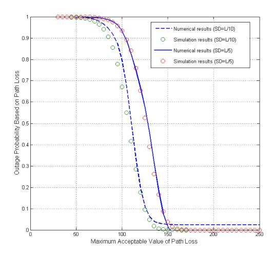
Figure 6.2: Outage probability based on PL threshold for different standard deviation of Gaussian distributed users in a circular cell
