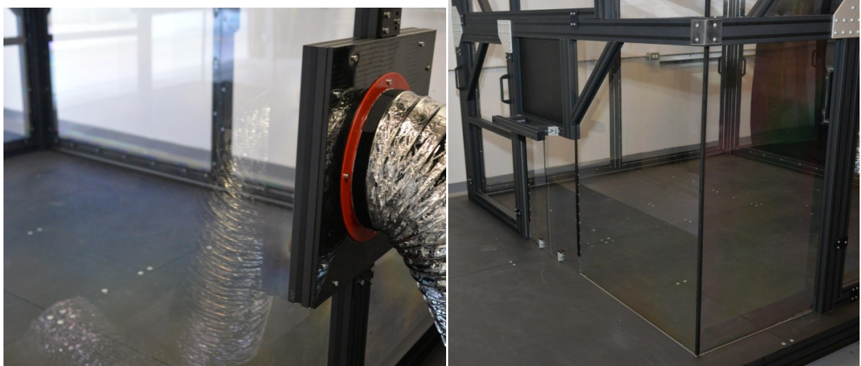
Figure 70. The fan duct (right) and the PIV clear corner of the CUBE (pictures provided by MĚKANIC)
