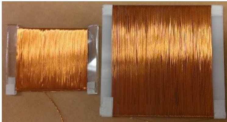
Fig. 3.16 Two H -coil sizes of 30 mm by 30 mm by 1.4 mm of 180 turns, and 53 mm by 44 mm by 1.6 mm of 220 turns
