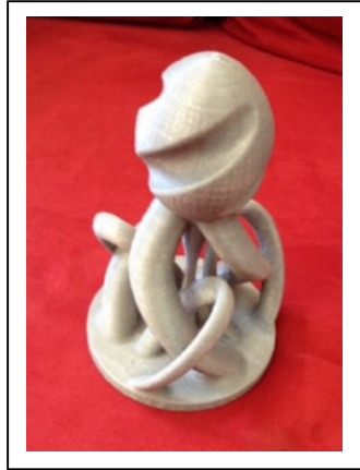
Figure 1-5: An example of a very complex 3D printed structure that would be very expensive (if not impossible) to make using conventional machining. 3
