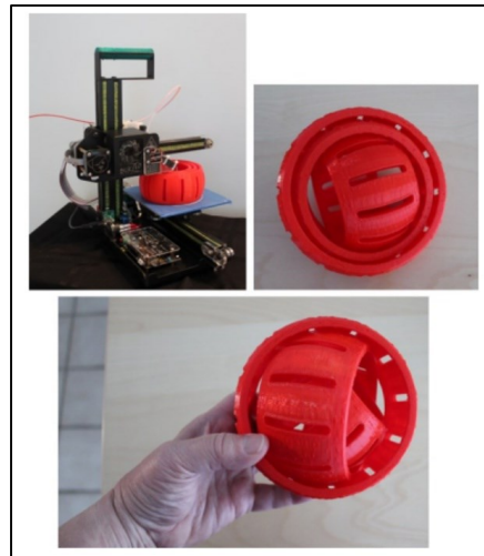
Figure 1-6: An example of an assembly with moving parts printed all in one shot. 3
