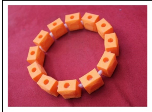
Figure 1-7: An example of a part made of two different materials (the orange, rigid, and the purple, flexible) printed at one shot. 3
