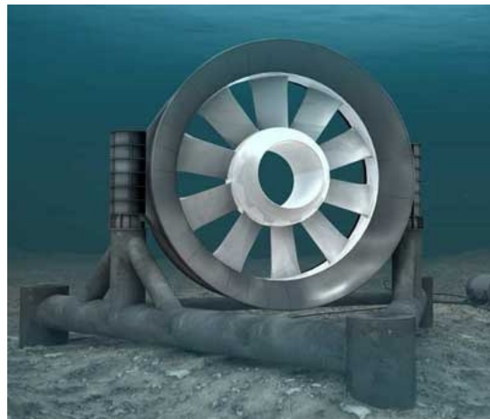
Figure 1.2. OpenHydro open-centre turbine (OpenHydro, 2015)
