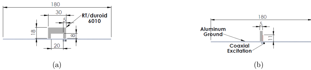
Figure A.6: The U-Shaped DRA structure (dimensions in millimeter). (a) Front view. (b) Side view.
