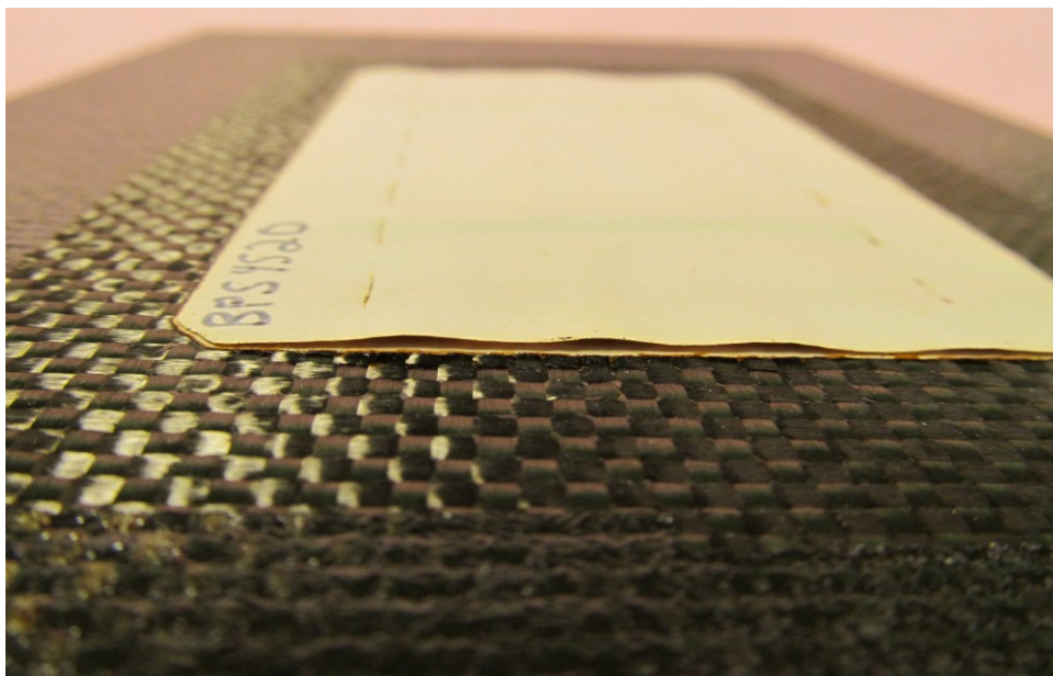
Figure 5-15 – Carbon fibre/BMI (BPS 4520) Panel: Label Delamination
