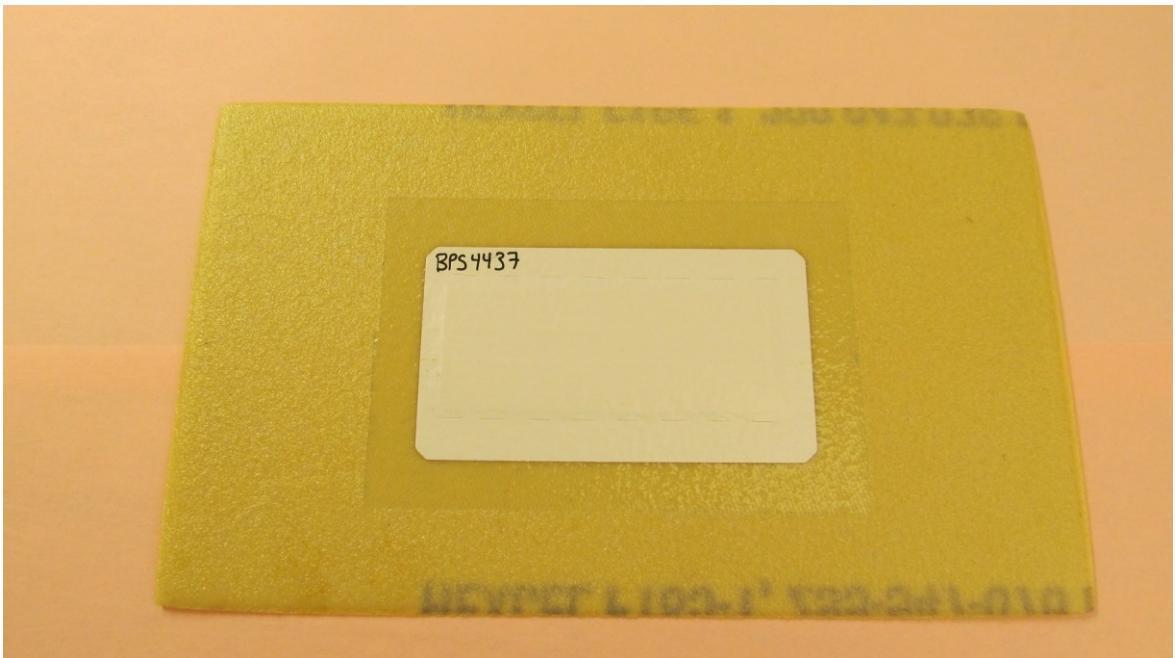
Figure 5-9 – Glass fibre/epoxy coupon (BPS 4437)
