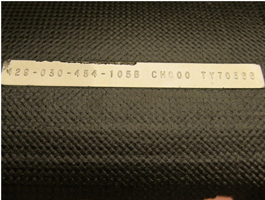
Figure 5-1: Traditional Embossed Aluminium Tape
