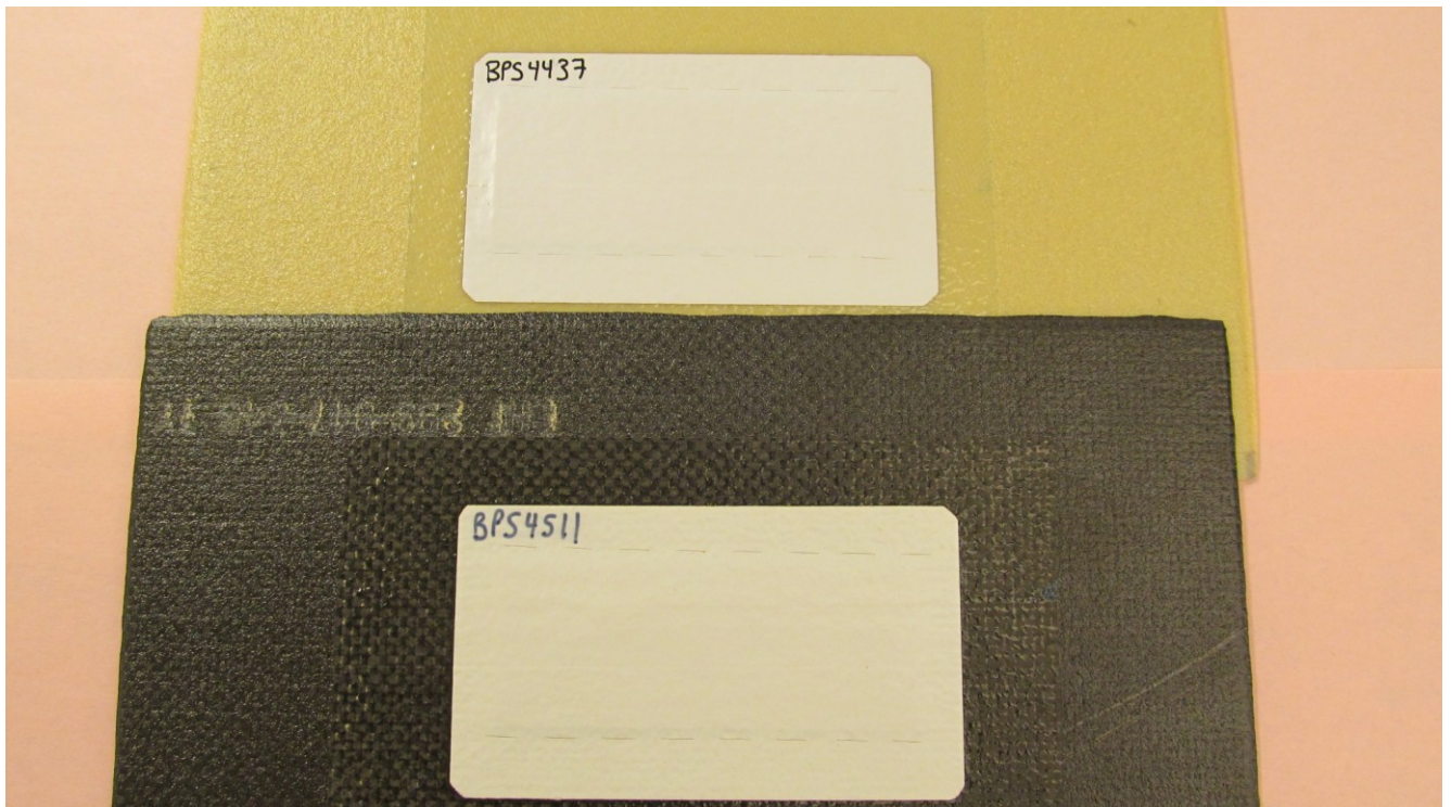
Figure 5-13 – Carbon fibre/Epoxy (BPS 4511) vs. Glass fibre/Epoxy coupon (BPS 4437)
