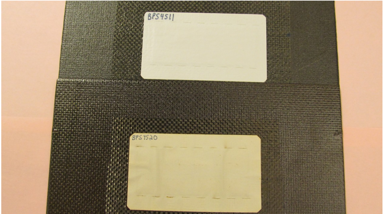
Figure 5-12 : Carbon fibre/BMI (BPS 4520) vs. Carbon fibre/Epoxy coupon (BPS 4511)
