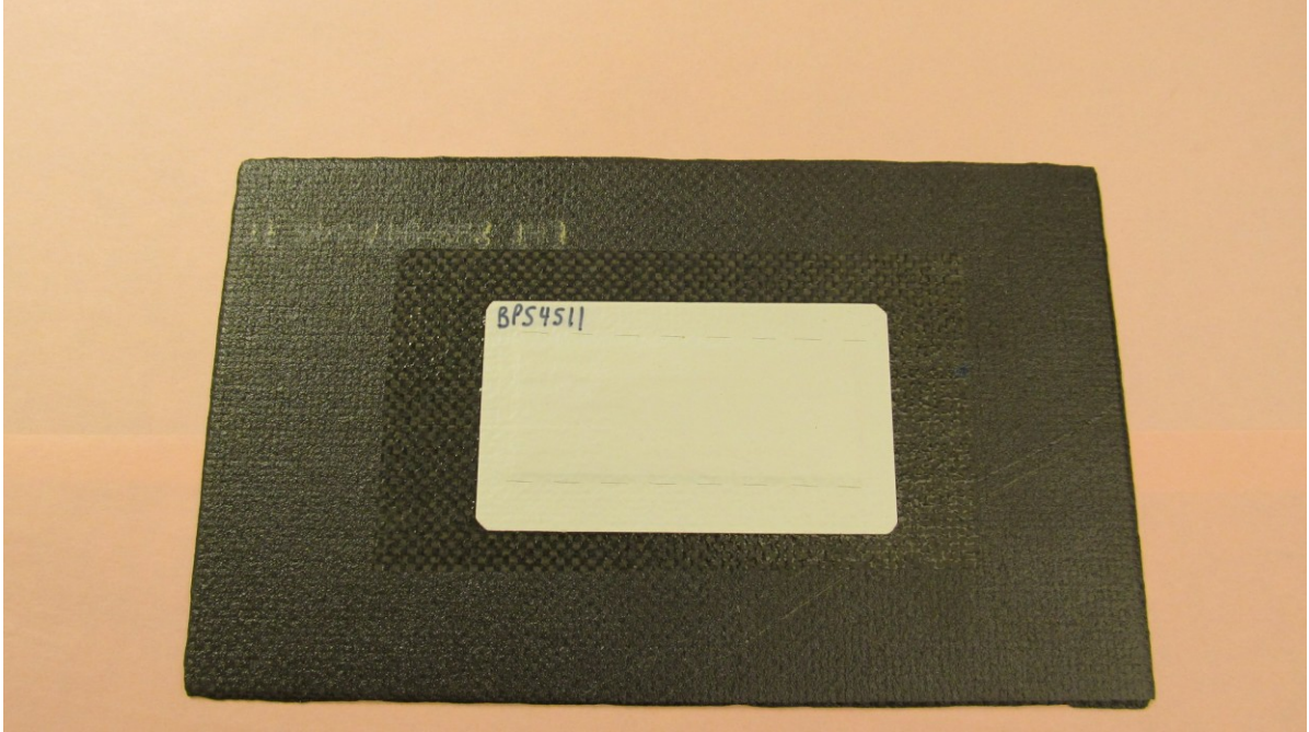
Figure 5-10 – Carbon fibre/Epoxy coupon (BPS 4511)
