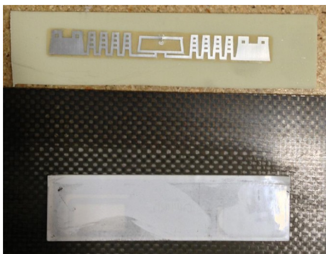
Figure 2-6 – RFID Tag and Inlay (comprising antenna and computer chip (memory))
