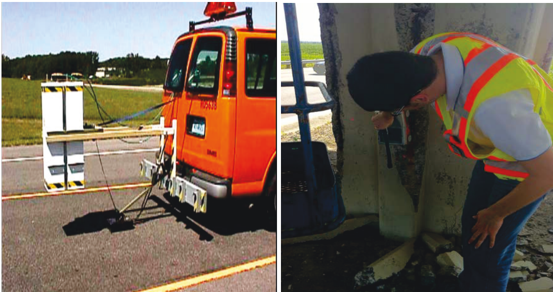
Figure 2-5 A) GPR air-coupled machine (Al-Qadi 2003). B) Handheld GPR machine
