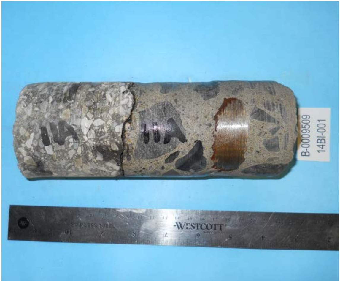
Figure 5-26 Non-corroded coring sample
