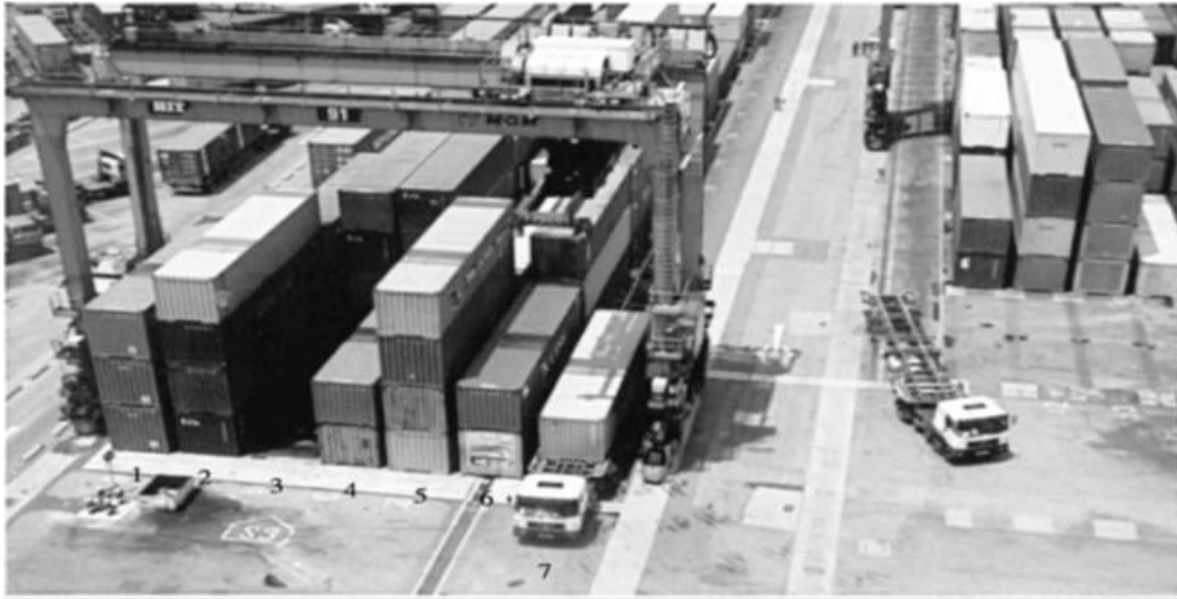
Figure 2- 4: An RTGC with width of 7 lanes; 6 for containers and the 7th for the trucks (Linn, 2003)
