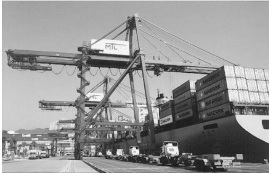
Figure 2- 5: Trucks arrive in a queue to be discharged or loaded by QCs (Linn, 2003)
