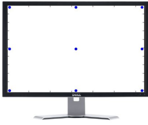
Figure 4.2 The 3-by-3 calibration grid on the screen.
