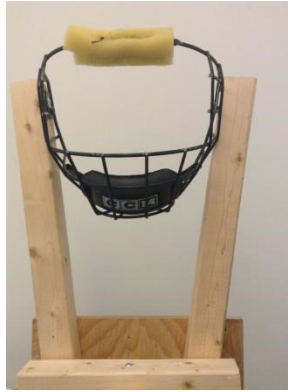
Figure 5.2 The headrest to restrict head movement.
