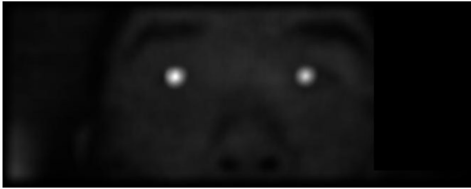
Figure 3.5 The normalized filtered image of Figure 3.3 with left pupil image as template image.
