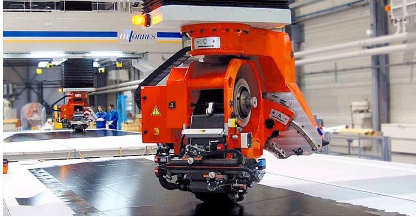
Figure 1.6 Automated Tape Laying (Photo Courtesy from Mtorres website) [8]
