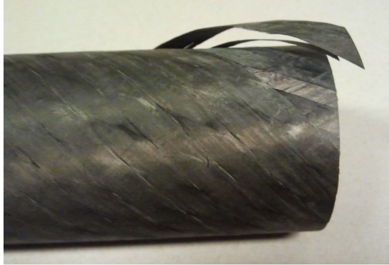
Figure 2.4 Poor bonding between layers of composite tube made by AFP
