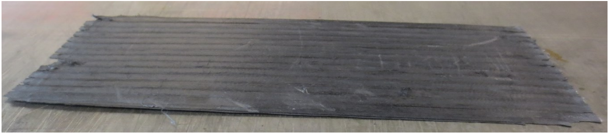
Figure 3.14 [0]_8 laminate after removing from mandrel
