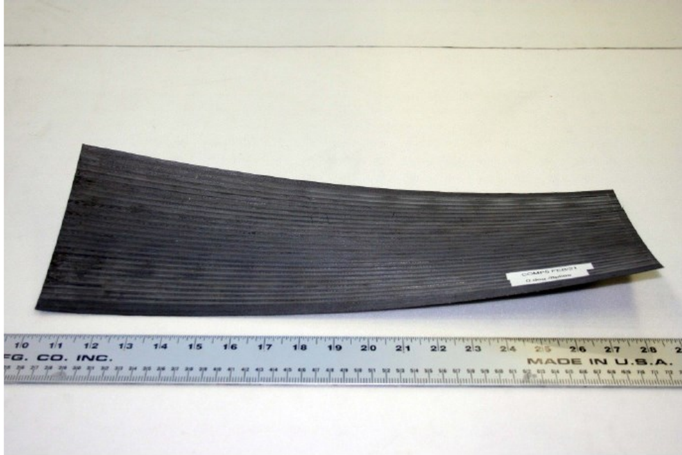
Figure 2.6 Illustration of warped laminate made by AFP[18]
