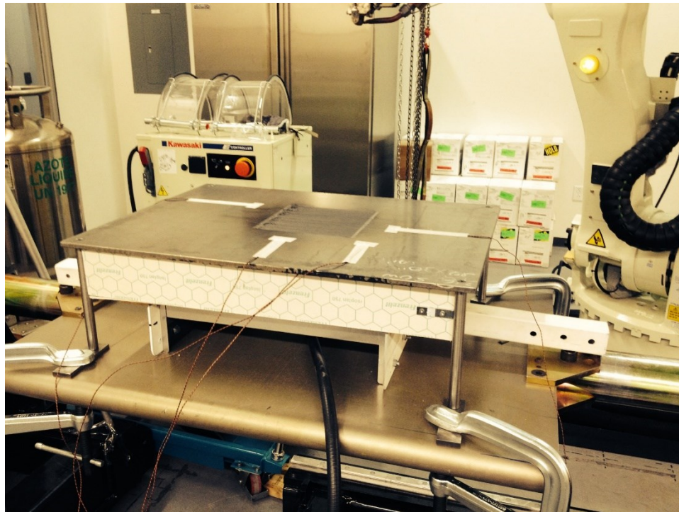
Figure 3.11 Heated mandrel setup
