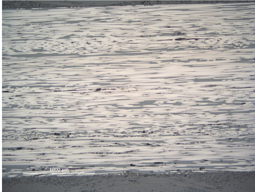
Figure 4.12 Microscopic image along fiber direction of [0]12 laminate made by AFP
