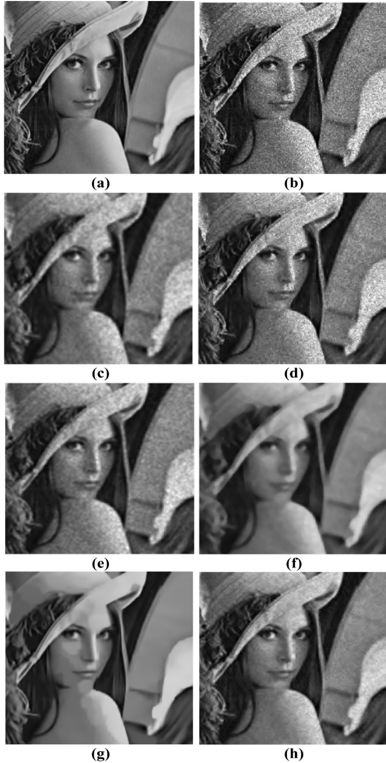
Figure 4.1: Magnified versions of the Lena image. (a) Original. (b) Noisy, M = 32 . Despeckled images using the (c) S-Threshold, (d) B-Shrink, (e) Lee-F, (f) SA-WBMAE, (g) SARBM3D, and (h) Proposed schemes.
