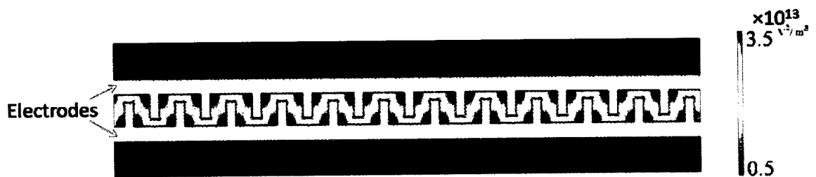
Figure 4.8: Numerical simulation for the distribution of DEP force between interdigitated electrodes ( 20\mu\text{m} electrodes, 30\mu\text{m} gap and 20 Volts peak-to-peak applied potential).
