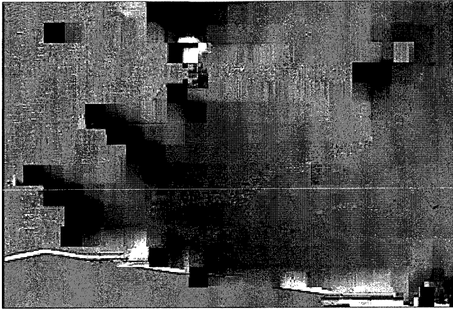
Figure 4.28: Frame 4 of video sequence “Table-Tennis” decoded using convolutional decoding only at channel SNR of 1.5dB.
