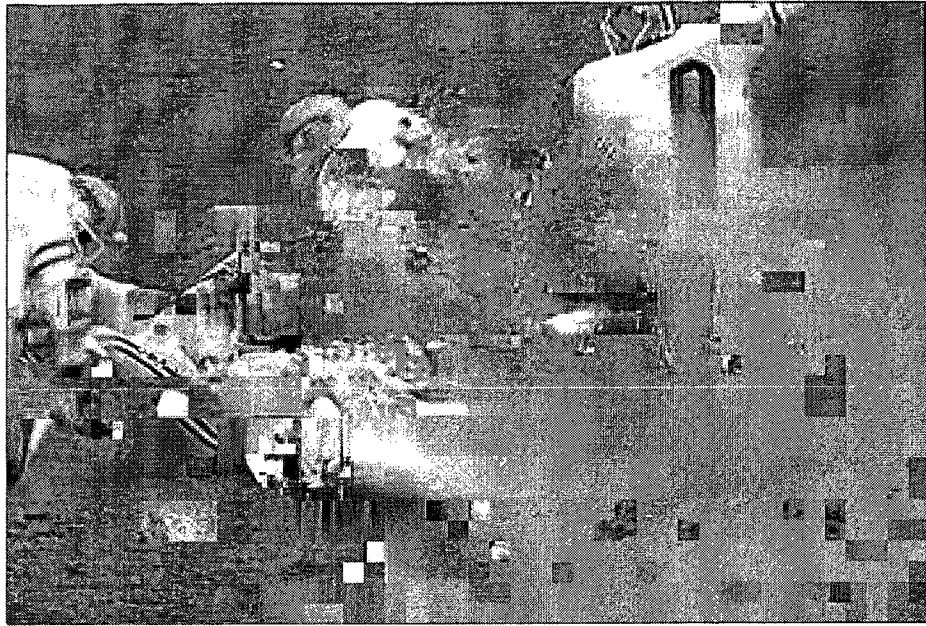
Figure 3.22: Frame 31 of video sequence “Football” transmitted over an AWGN channel at channel SNR of 1.8dB using convolutional decoding only.
