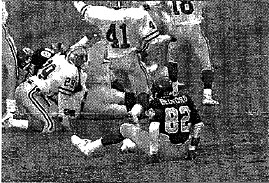
Figure 3.28: Frame 64 of video sequence “Football” decoded by the IJSCD-VC-PI scheme at channel SNR of 1.8dB and at the 4 th iteration.
