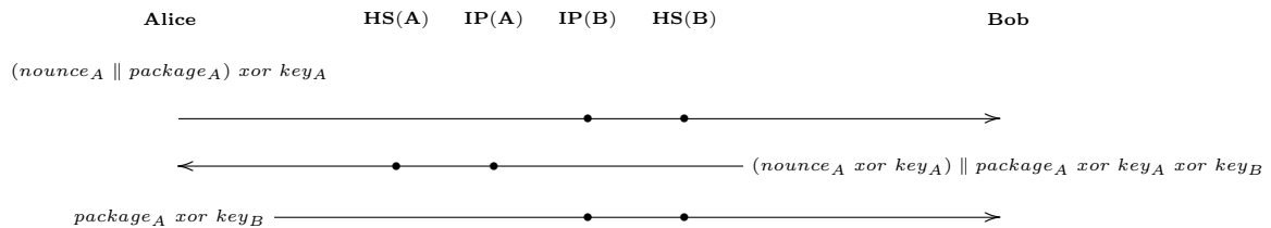
Figure 21: Secret sharing using Tor hidden service, Here, HS(A) and HS(B) are the hidden services of Alice, and Bob and IP(A) and IP(B) are introductory points of Alice and Bob respectively. Also, package_A = id_A \parallel cookie_A \parallel rp_A \parallel pubKey_A .
