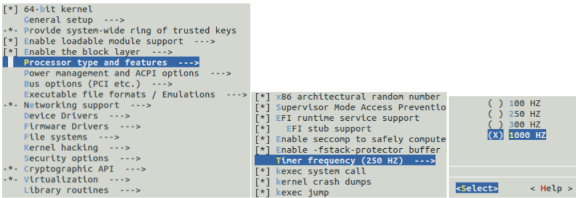
Figure 53. Kernel Timer Frequency Adjustment.
